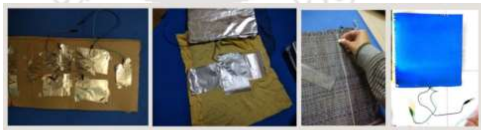
Figure 4. 6. Testing the stepping concept with Makey Makey: testing with foil with a sheet, cloth and finally on the floor mat from left to right: interface mat (initially used for the trial purpose)
