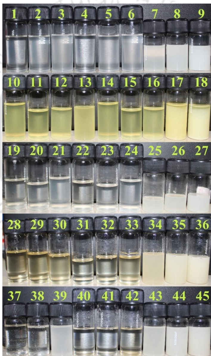
Figure 4.11: Visual observation of Prepared NDDES after 8 weeks (Numbers represent the NDDES from table 3.4)
