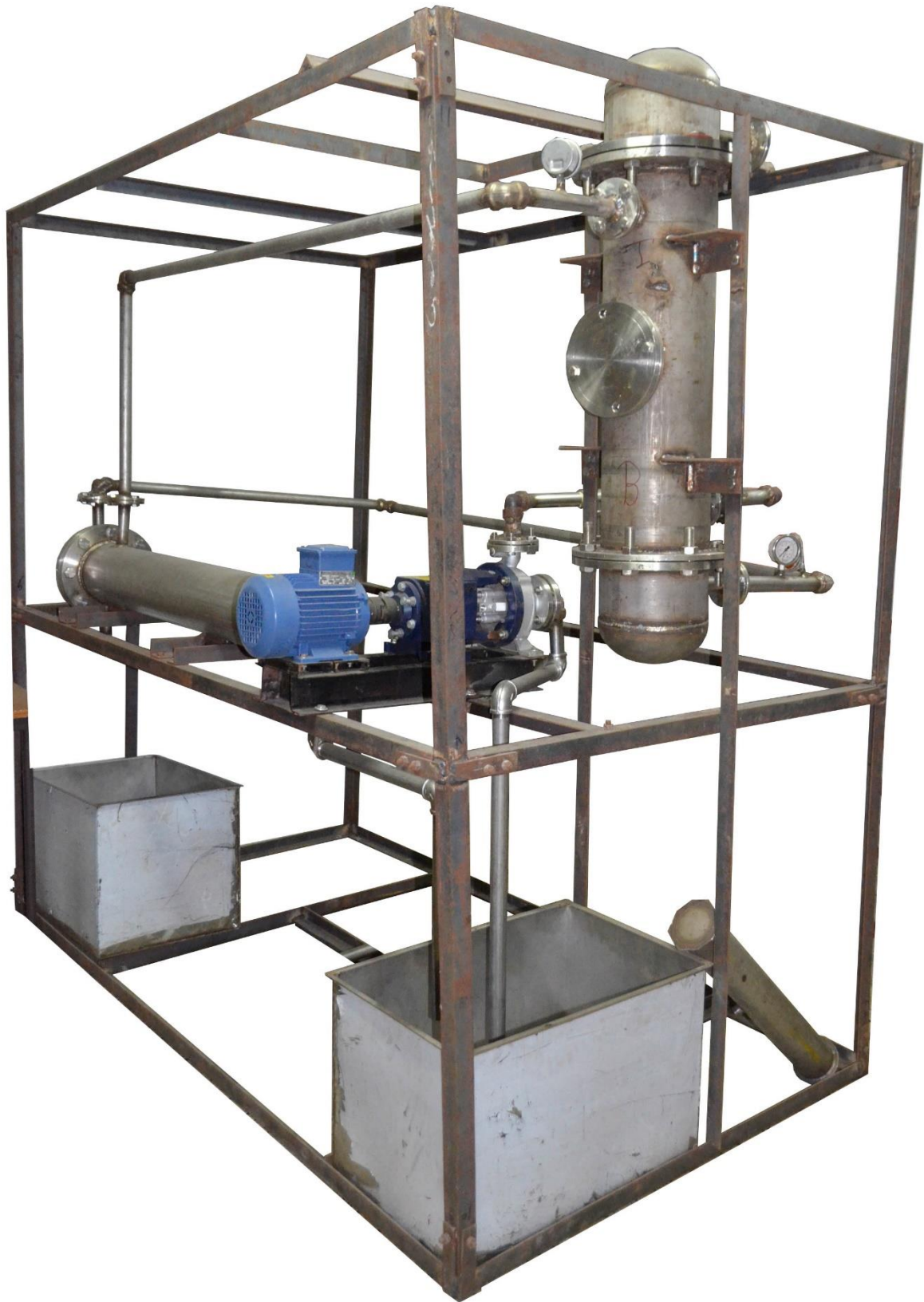
Steam Generation System
