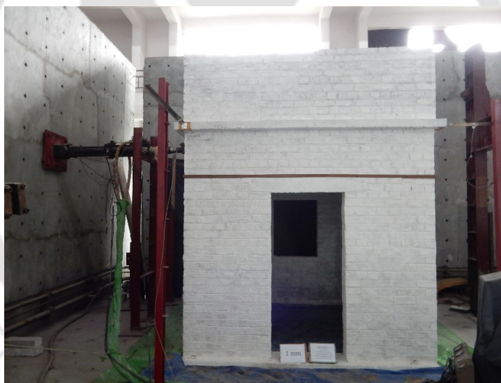
Figure 5.10. Experimental setup of strengthened URM building specimen 1 (Model 1).
