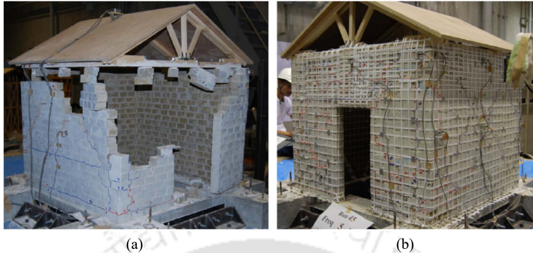
Figure 2.8. Effectiveness of polypropylene-band used as strengthening of URM building. Lateral load performance of (a) the unstrengthened model, and (b) the strengthened model (Sathiparan et al., 2012).
