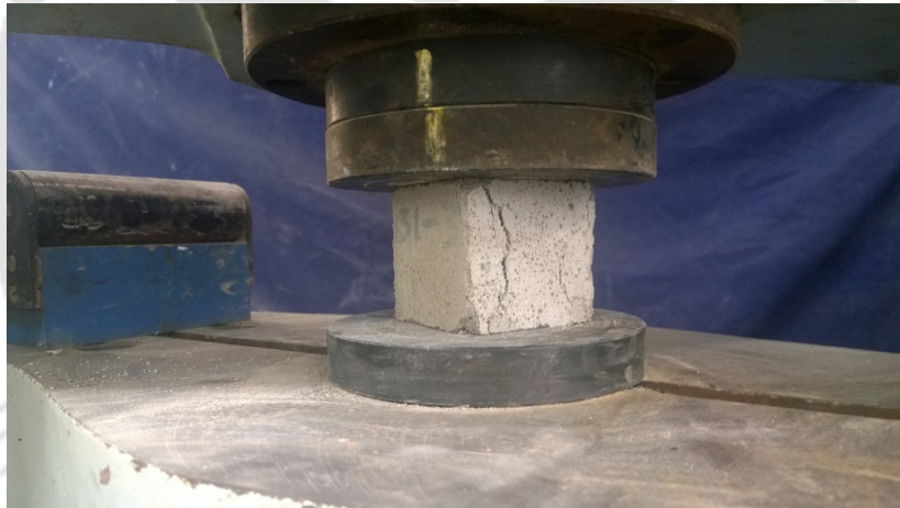
Figure 4.2. Compression test of cement mortar cubes.
