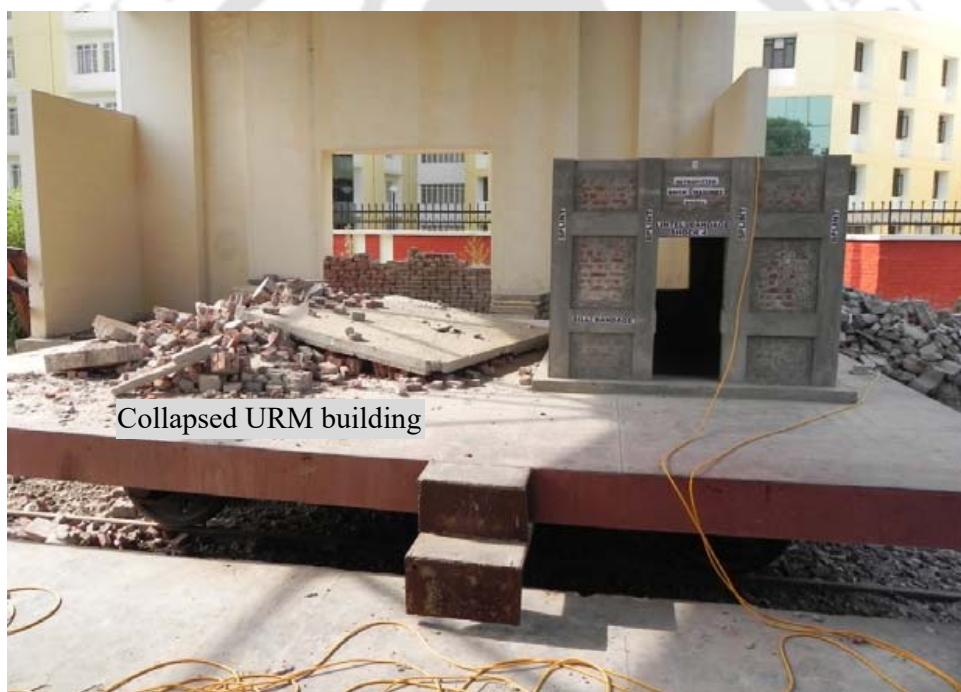
Figure 2.9. (a) Details of the ‘Splint and Bandage’ strengthening technique, and (b) shock-table test showing the effectiveness of using ferro-cement bands (welded wire mesh in concrete/mortar) applied on the URM walls as strengthening scheme. The building on the left was not strengthened, while the building on the right was strengthened using the ‘Splints and Bandage’ technique (Kadam et al., 2015, 2018).
