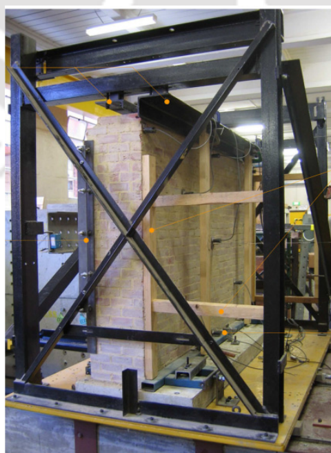
Figure 2.5. Out-of-plane test set up of URM wall (Vaculik and Griffith 2018).
