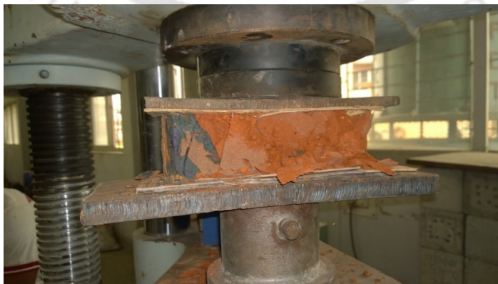
Figure 4.1. Compression test of bricks.
