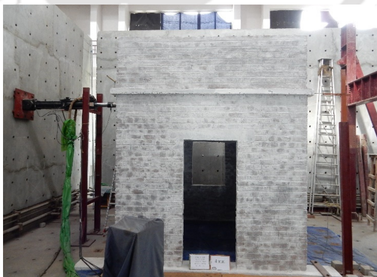
Figure 5.6. Experimental setup of URM building.
