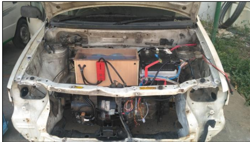
Figure 4.27: Installation of the SC bank in the EV-II
