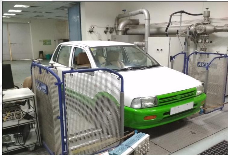
Figure 5.5. Test setup and road load simulation test of the EV-II on the chassis dynamometer.
