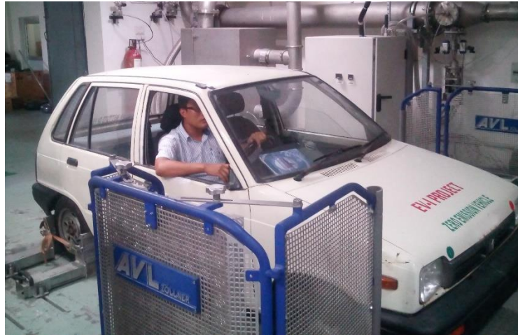
Figure 5.4. Road load simulation test of the EV-I on the chassis dynamometer
