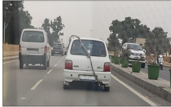
Figure 3.12: Pitot tube setup on the in-use ICE car
