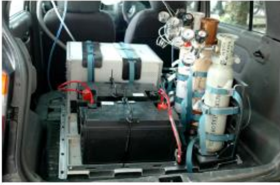
Figure 3.11: PEMS inside the in-use ICE car
