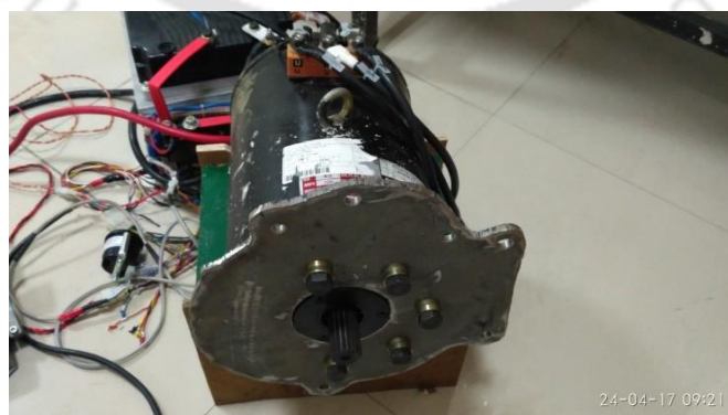
Figure 4.7: Adaptor plate integration with the EM.
