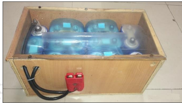
Figure 3.5: Integrated Supercapacitor Bank
