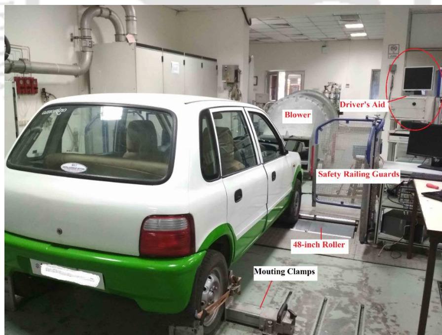
Figure 3.6: Test cell description with a test vehicle mounted on the chassis dyno.
