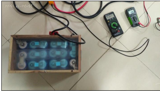
Figure 4.23: Charging of the SC Bank.
