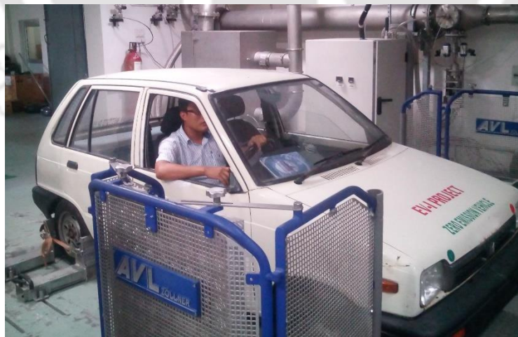
Figure 3.17. Road load simulation test of the EV-I (before repaint) on the chassis dynamometer
