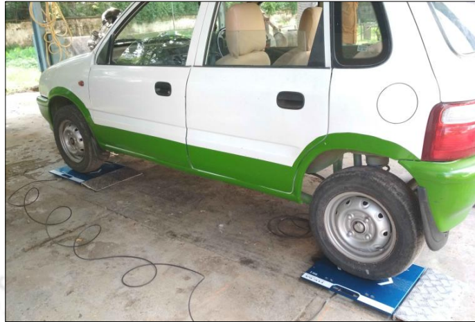
Figure 3.10. Digital vehicle weighing for the test vehicle
