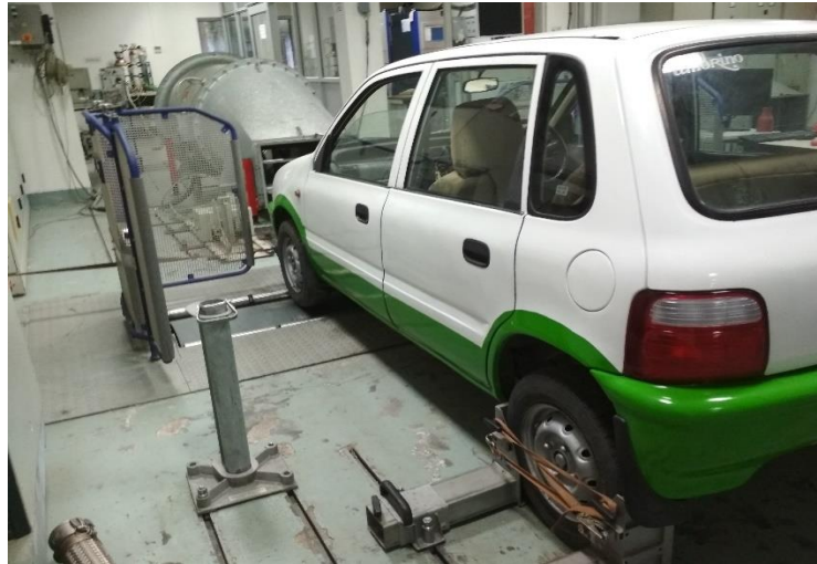
Figure 3.18. Setup of test vehicle EV-II on the Chassis Dynamometer
