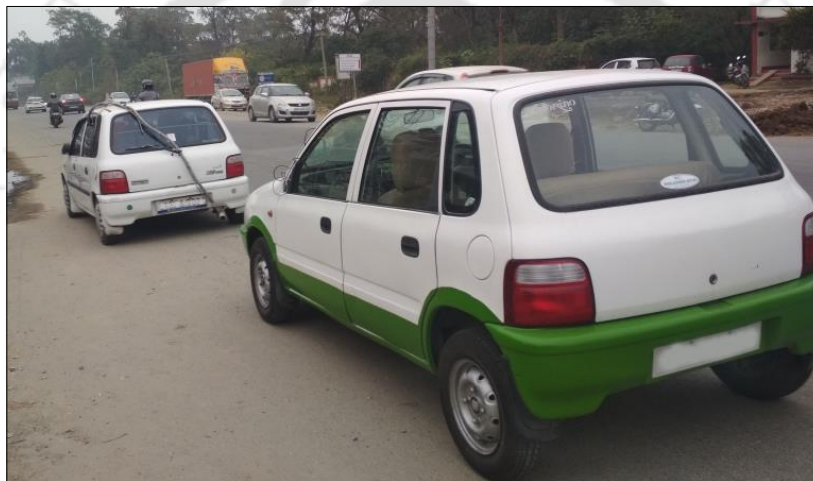
Figure 6.1. Car chasing technique for the real-world tests
