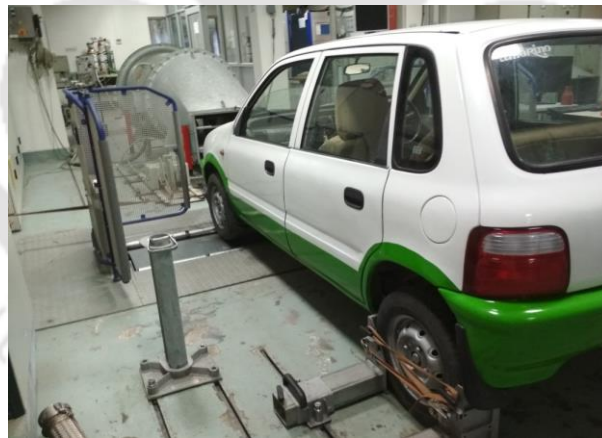
Figure 1.6: EV-II set up in the chassis dynamometer laboratory
