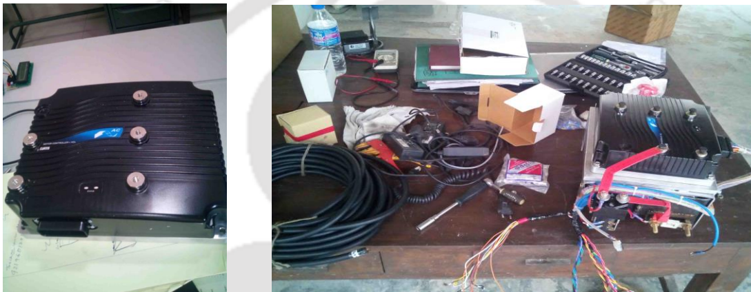
Figure 4.15: Curtis motor controller and wiring-harness
