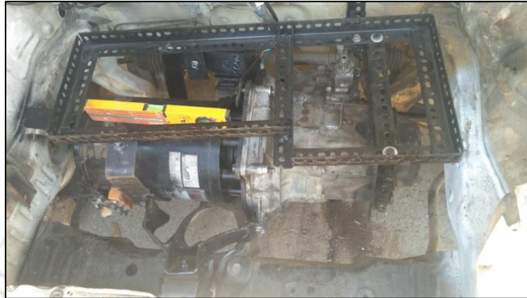
Figure 4.9: Motor mounting and base frame for the electrical subsystems
