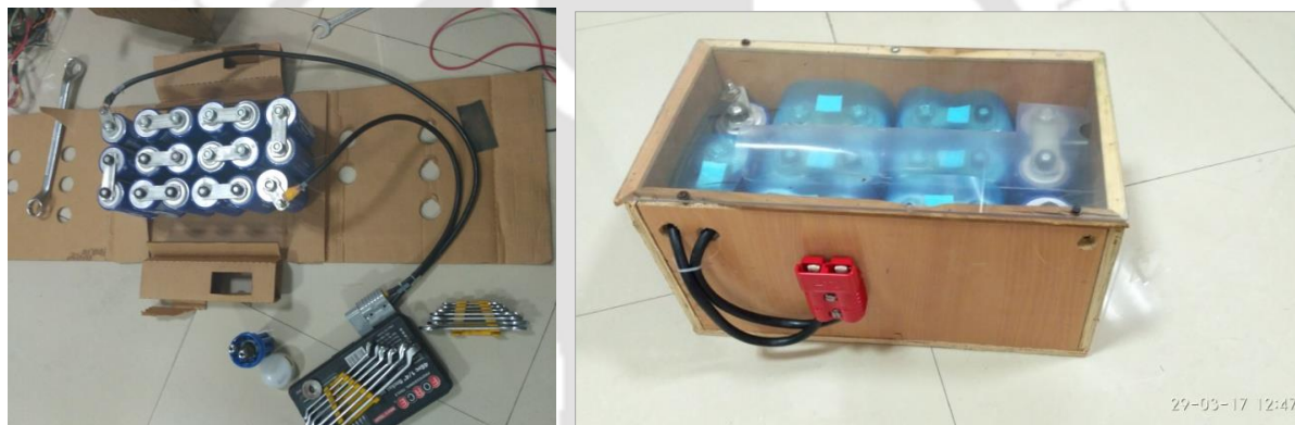
Figure 4.22: An integrated SC bank of 48V, 189F.
