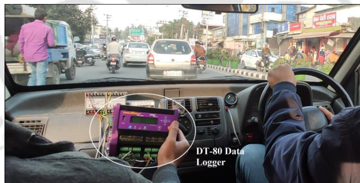
Figure 3.19. The actual setup of the GPS data logger inside the test car
