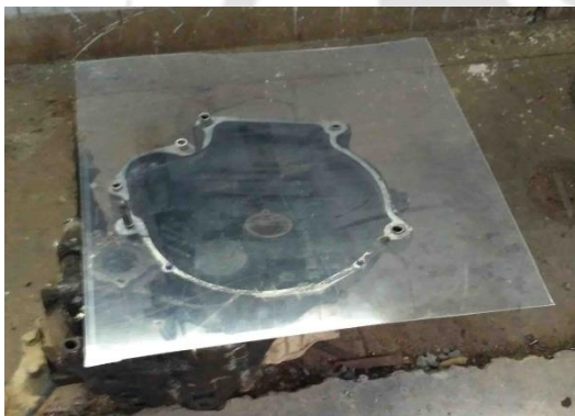
Figure 4.5: Template development for the adaptor plate.
