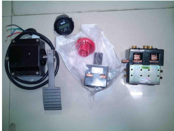
Figure 4.16: Foot Pedal, Disconnect switch, BDU, F/R Contactor
