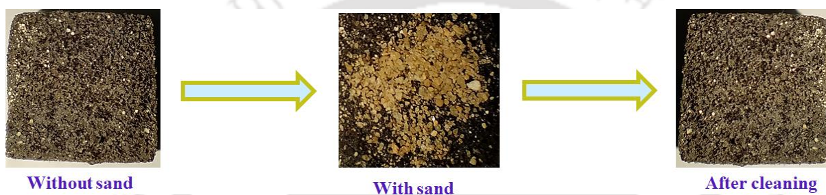
Figure 5.44 Digital image of 4'@CF 3 @melamine composite displaying self-cleaning nature.
