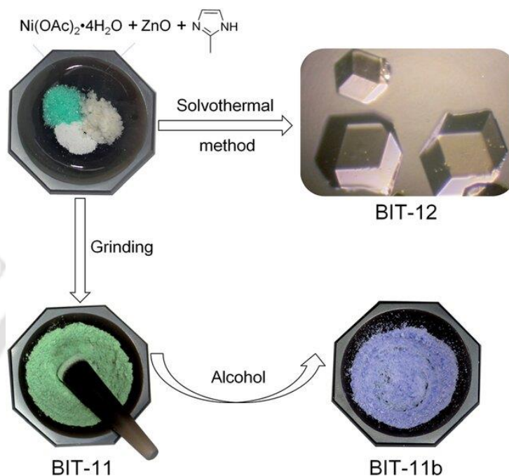
Figure 1.10 Schematic representation of the mechanochemical synthesis of BIT-11 and BIT-11b, as well as the microscopic photo of BIT-12 single crystals synthesized solvothermally. This image is collected with permission from ref. no. 118. Copyright 2014, Royal Society of Chemistry.
