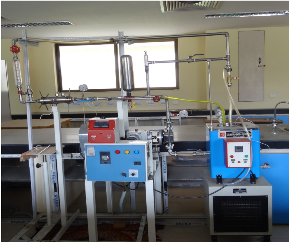
Figure G3: Cross flow Microfiltration Setup (Courtesy: Department of Biotechnology Juice Clarification Project)
