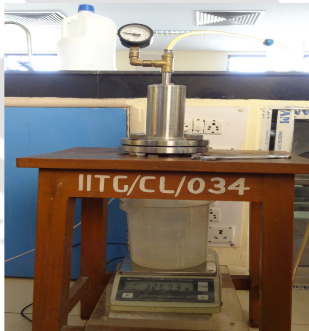
Figure G2: Dead end Microfiltration Setup
