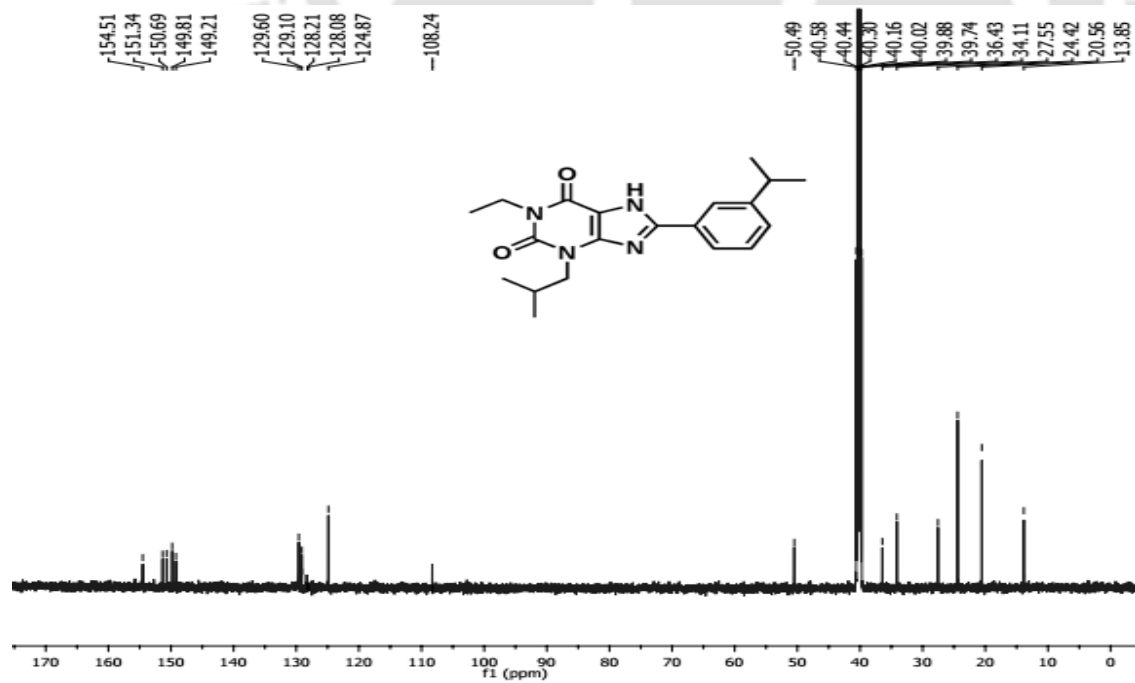
Figure A1.52 13 C NMR (DMSO-d 6 ; 150 MHz) spectra of compound 6a5 or C5
