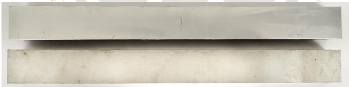
Figure 6.8 Photograph of the fabricated tensile test specimen Al 6061-T6 (top) and SS 316 (bottom)
