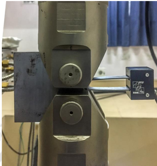
Figure 6.10 Mode I CT specimen with the COD gauge for fatigue test
