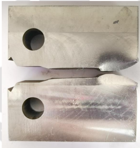
Figure 8.2 Fractured CT specimen made of SS 316
