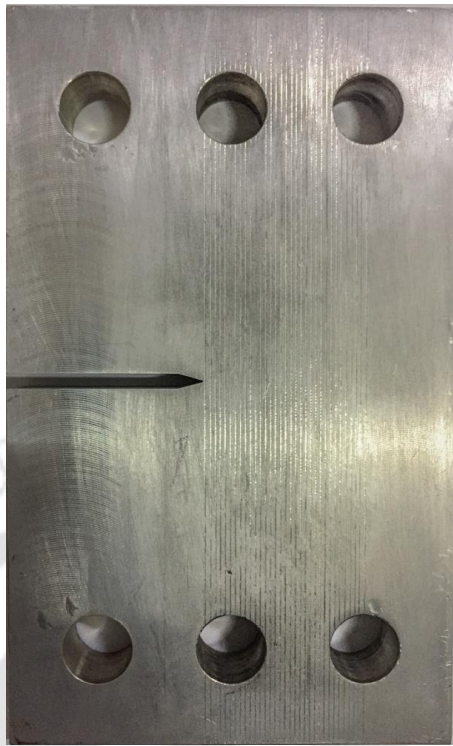
Figure 6.13 CTS specimen with the grid lines
