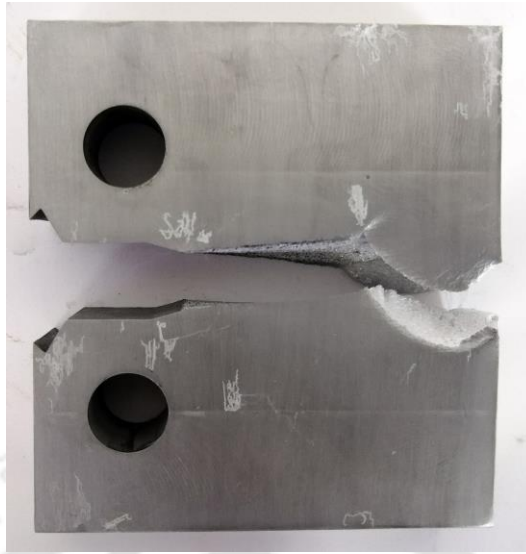
Figure 7.2 Fractured mode I specimen made of Al 6061-T6 alloy
