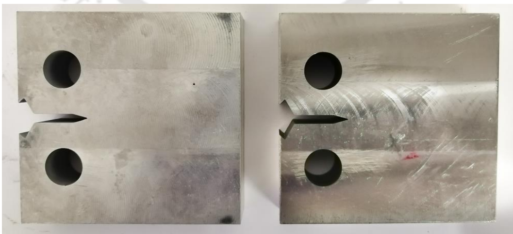
Figure 6.6 Photograph of the fabricated CT specimen Al 6061-T6 (left) and SS 316 (right)
