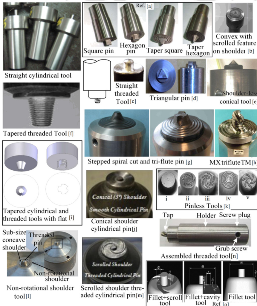
Figure 2.3 FSW tool geometries
