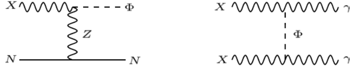
Figure 6.10: Left: Inelastic DM scattering off the nuclei N for direct search of DM; right: DM annihilating to photon final states via \Phi mediation for indirect search of DM.
