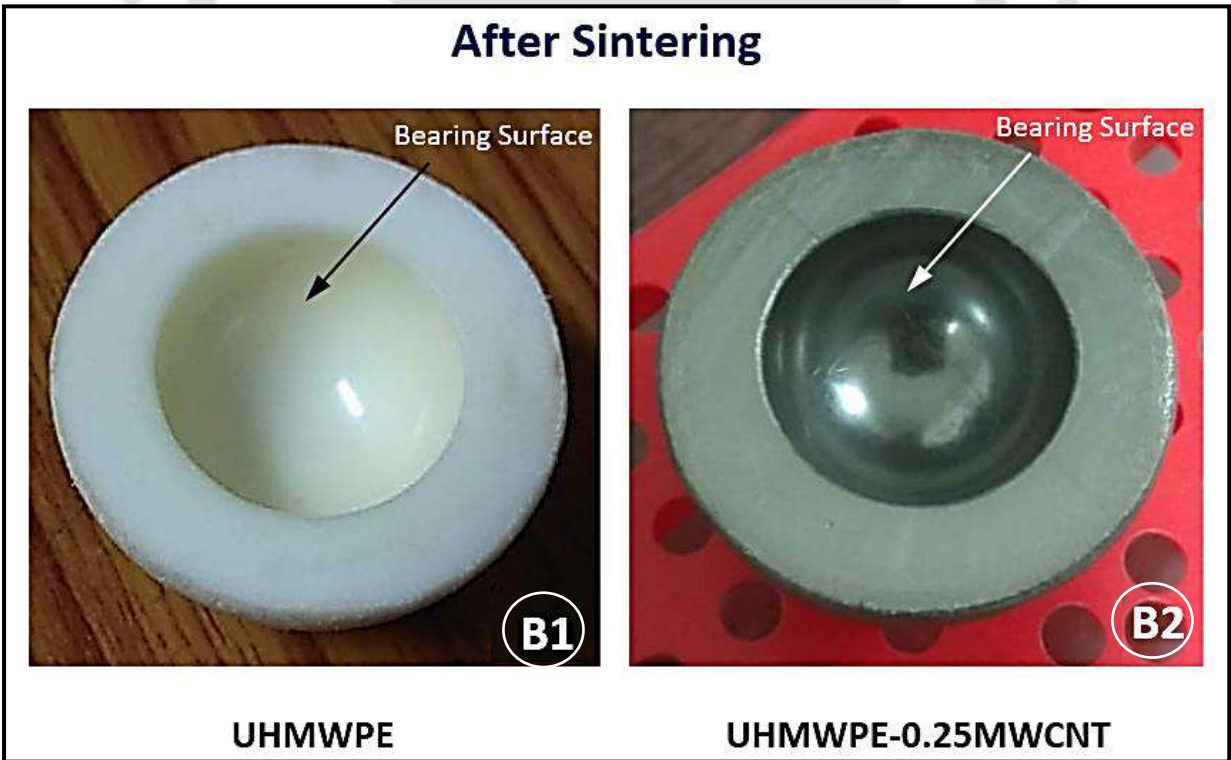
Figure 4.5.(A1) UHMWPE powder after compacted in acetabular liner shape (A2) UHMWPE-0.25MWCNT powder mixture after compacted in acetabular liner shape (B1) UHMWPE liners finally obtained after sintering (B2) UHMWPE-0.25MWCNT liners finally obtained after sintering without any machining or finishing operation.
