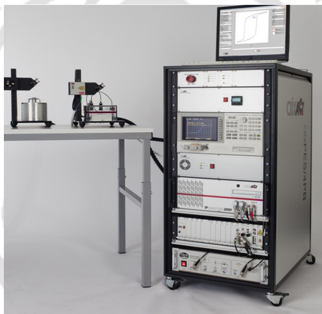
Figure 2.14: Photographic view of the ferroelectric polarization-electric field tester.
