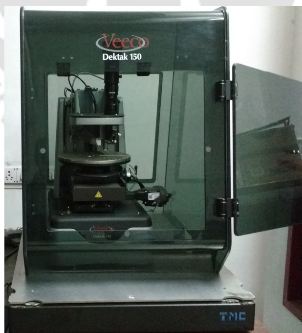
Figure 2.16: Photographic view of the stylus profilometer.
