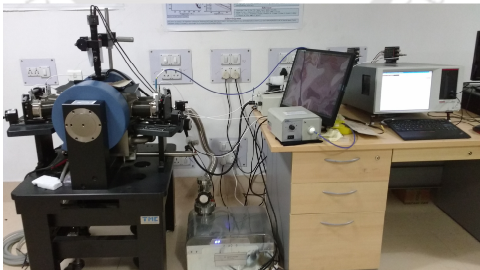
Figure 2.22: Photographic view of the Keithley 4200 semiconductor systems along with probe station.
