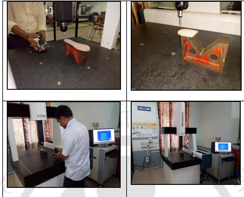
Figure 4. 8: Sole profile measurement on CMM
