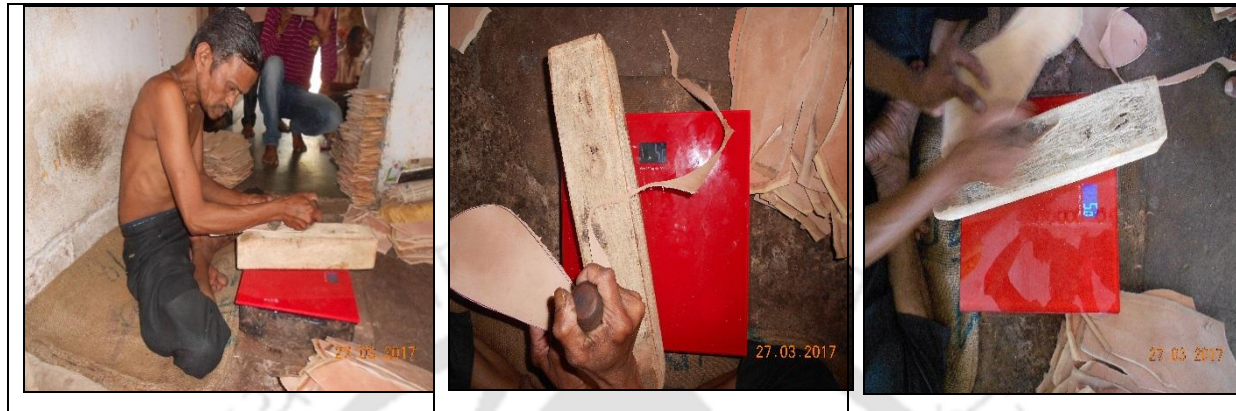
Figure 3. 2: Measurement of force required for sole cutting activity
