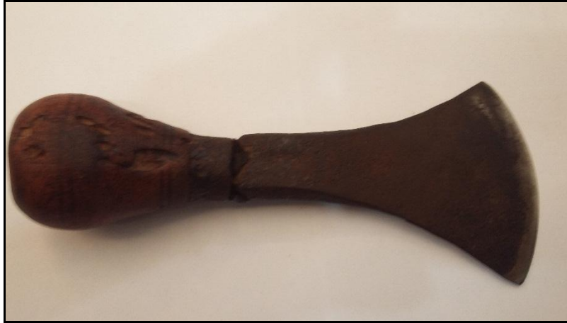
Figure 4. 4: Rappi (sharp-edged tool) tool used for sole preparation
