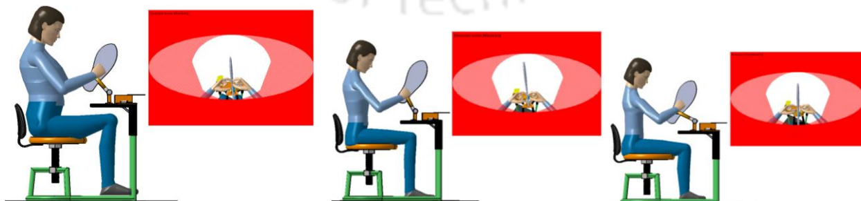
Figure 5. 8: Vision analysis of 95 th percentile, 50 th percentile and 5 th percentile of female
