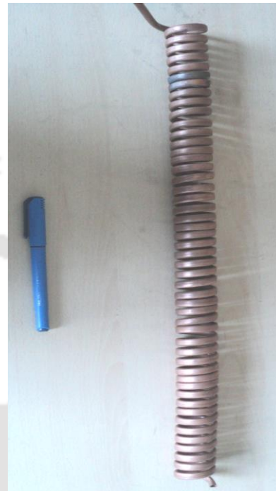
Fig. 3.9 Photograph of the copper coil used in the heat exchanger
