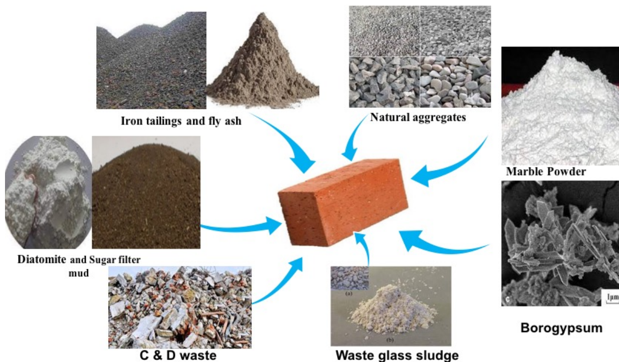
Figure 1 - 2 Inorganic wastes recycled into fired brick production
