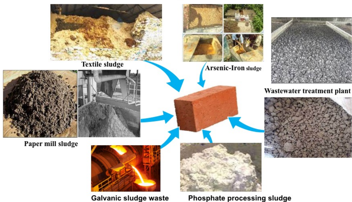
Figure 1 - 3 Sludge incorporated in fired brick making
