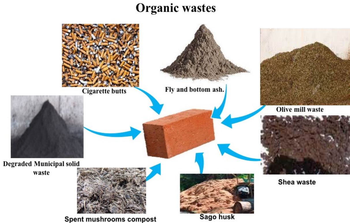
Figure 1 - 1 Different organic wastes recycled into fired brick manufacturing
