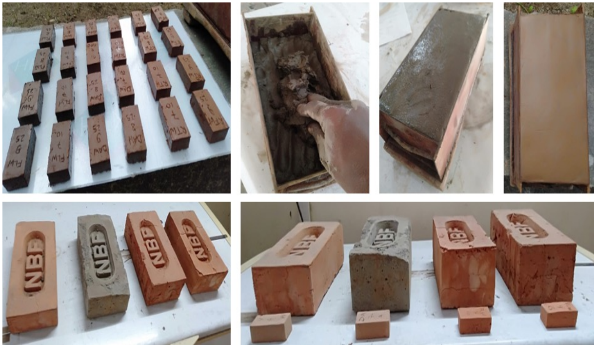
Figure 6- 1 Laboratory and commercial sized fired brick manufactured with incorporation of waste at three different temperatures
