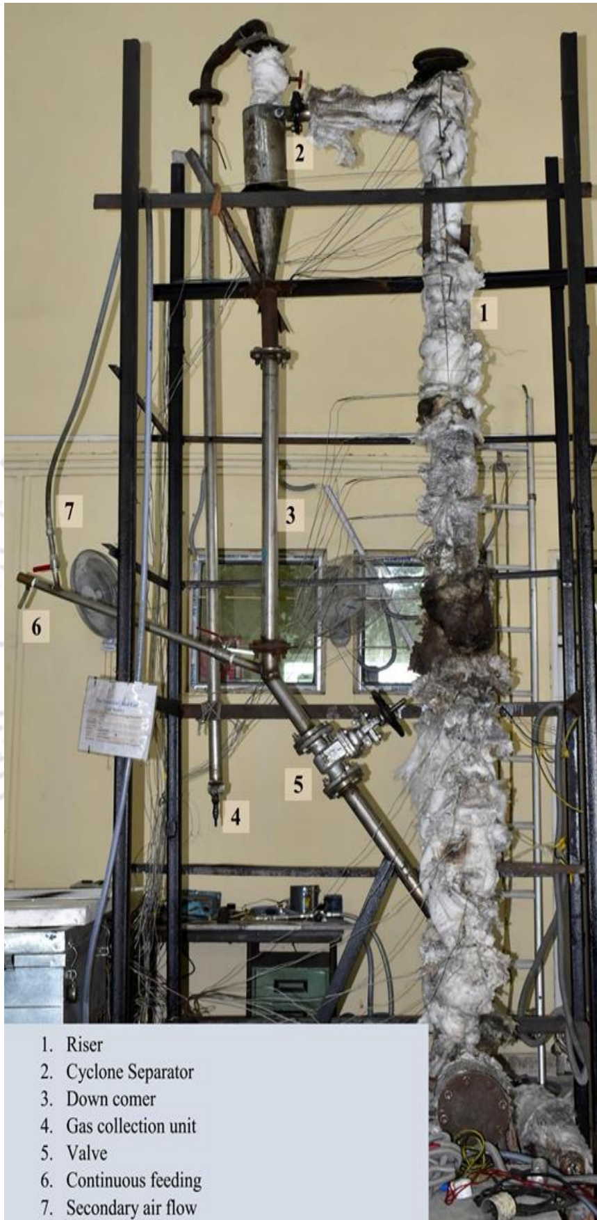
Fig. 4.2 Photograph of the PCFB experimental setup
