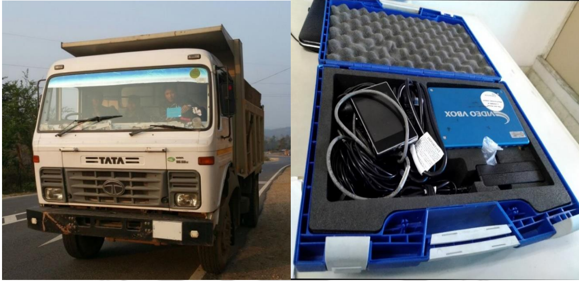
Fig. 3.7 Test vehicle (2-axle empty truck) equipped with V-Box
