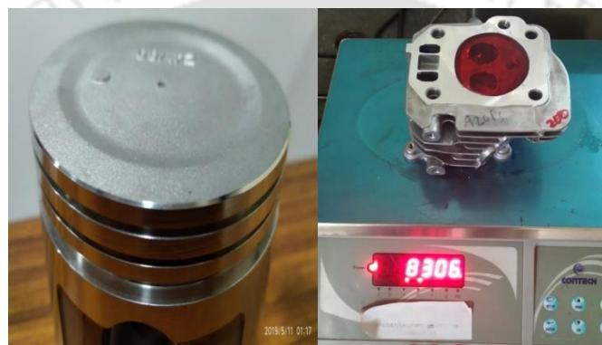
Fig. 3. 26: Measuring technique of piston cavity and combustion chamber volume: Honda GX 200
