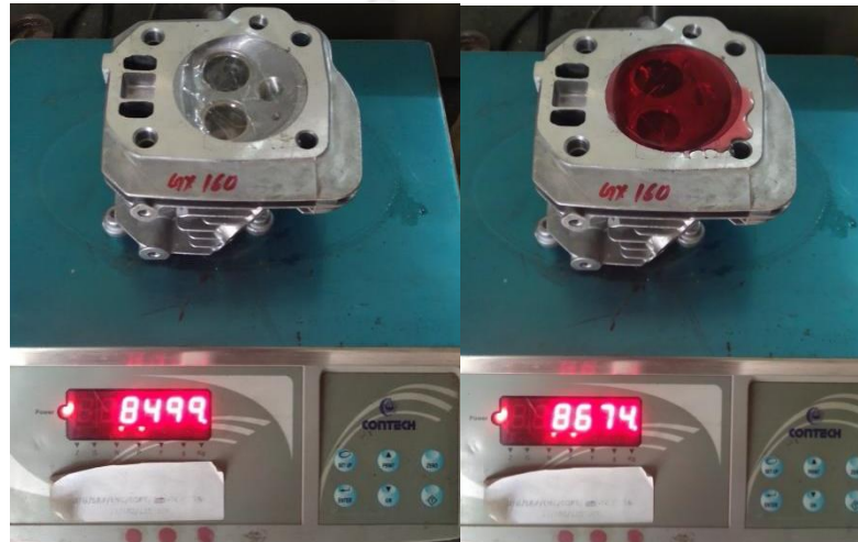
Fig. 3.27: Measuring technique of combustion chamber vol.: Honda GX 160 engine head
