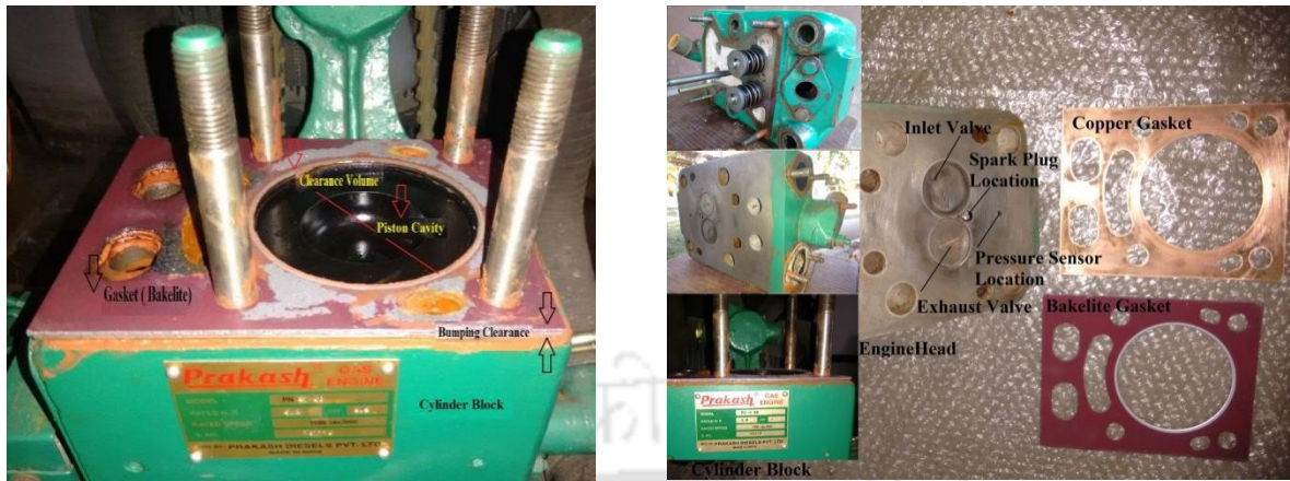
Fig. 3. 3: Engine cylinder Block and head with CR variation attachments
