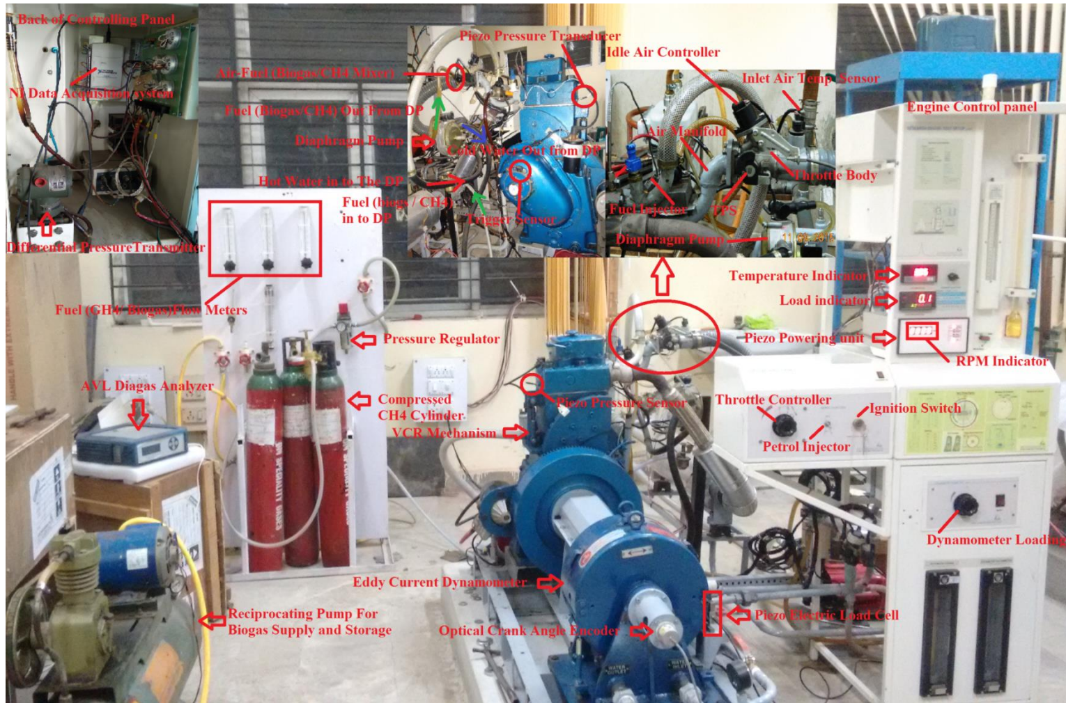
Fig. 3. 6: Pictorial representation of the VCR SI research engine test facility
