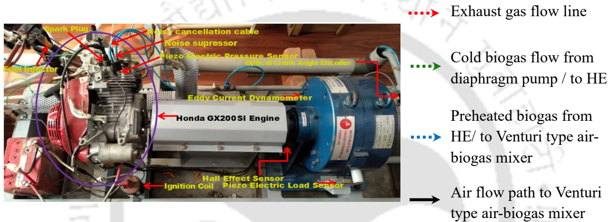
(a) Mounted instruments on biogas fueled retrofitted Honda GX 200 SI engine test rig
