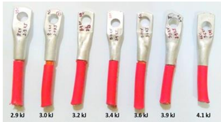
Figure 3.8 EM crimped samples at various discharge energy
