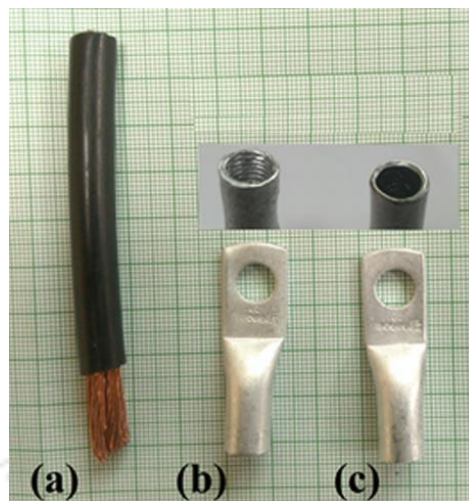
Figure 4.14 (a) 25 mm 2 copper wire, (b) Internal threaded terminal, and (c) Plain terminal
