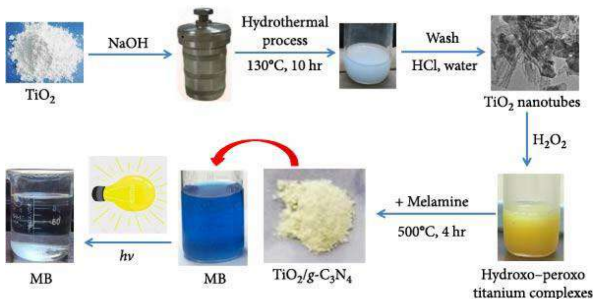
Figure 1.8: Schematic synthesis route of chemical-based \text{TiO}_2/\text{g-C}_3\text{N}_4 and photocatalytic degradation of MB dye (Reprinted with permission from (Hoa et al., 2023), Copyright 2023 Dang Thi Ngoc Hoa et al.).
