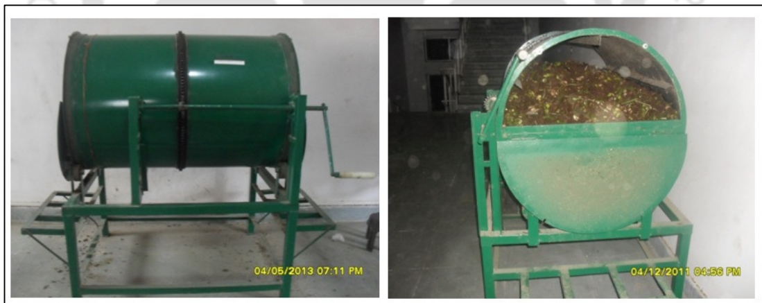
Fig. 3.8 Schematic diagram and pictorial view of a rotary drum composter for batch operation
