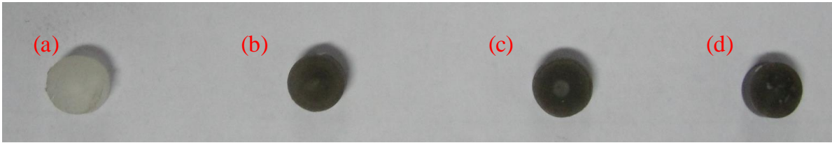
Figure 2.13 (a) Polypropylene, (b) 5%, (c) 10% and (d) 15% cement filled composite samples
