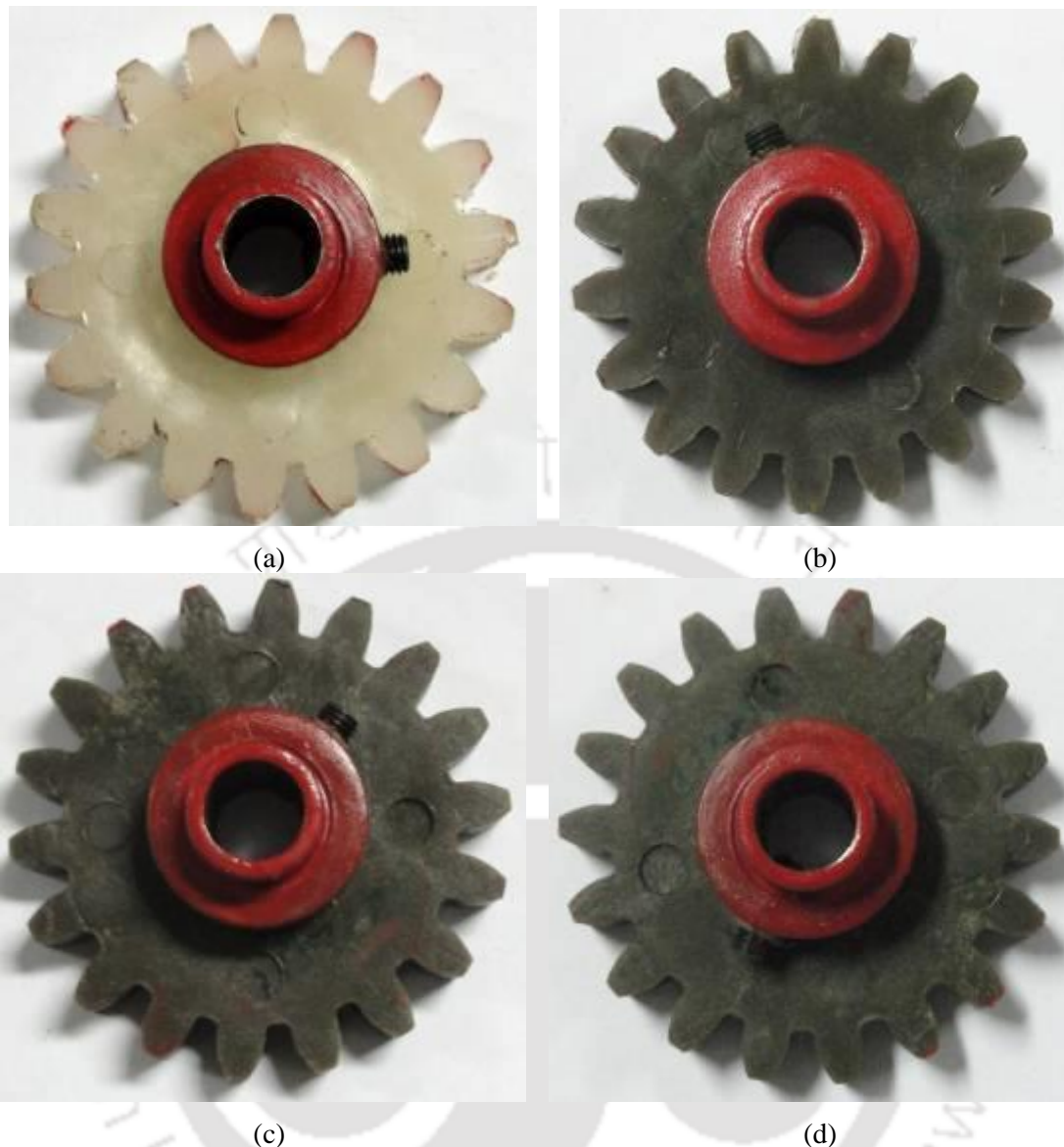
Figure 5.1 Fabricated composite gears with bush (a) pure polypropylene, (b) 5%, (c) 10% and (d) 15% cement reinforced composite spur gears
