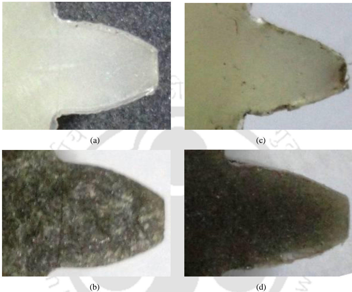
Figure 5.30 Intact tooth profile of (a) pure polypropylene, (b)10% cement filled composite and tooth profile after test (c) pure polypropylene, (d) 10% cement filled composite gears
