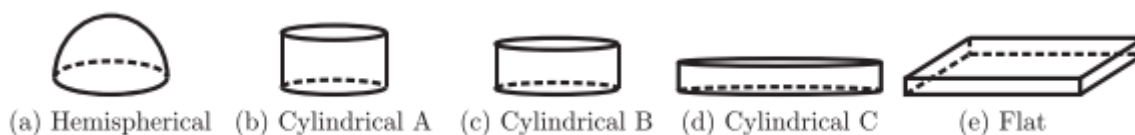
Fig. 2.3. Generic shapes of the high-explosives used in the numerical models: (a) hemispherical, (b-d) cylindrical and (e) flat (Artero-Guerrero et al., 2017).
