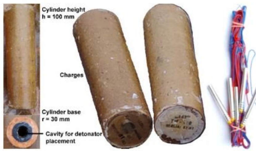
Fig. 2.2. Charge geometry and detonator capsules filled with lead azide (LUKIĆ et al., 2020).
