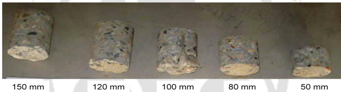
Figure 3.16: Core samples collected from test sections show good compaction and thickness of each section is maintained properly.
