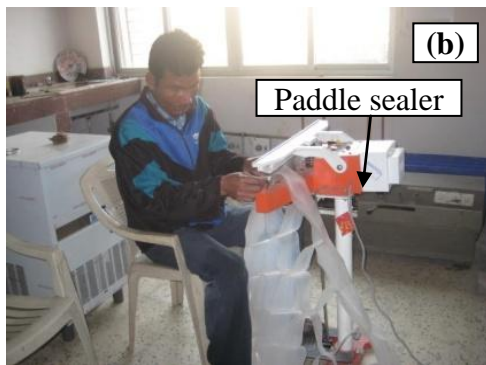
Figure 3.1: a) Low Density Polyethylene (LDPE) pipe (0.49 mm thick and 101.6 mm in diameter), b) Sealing of plastic cell formwork using paddle sealer, and c) Finished plastic cell formwork of pocket size 150 mm x 150 mm.
