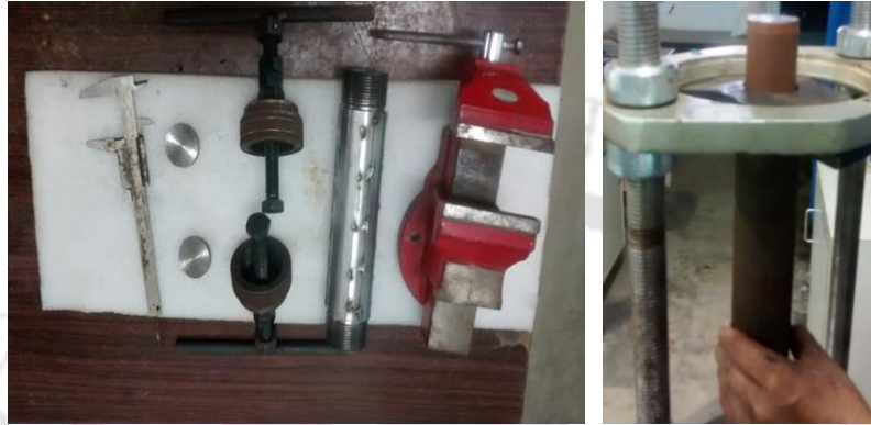
Figure 3.29 Unconfined compression test sample preparation and extraction
