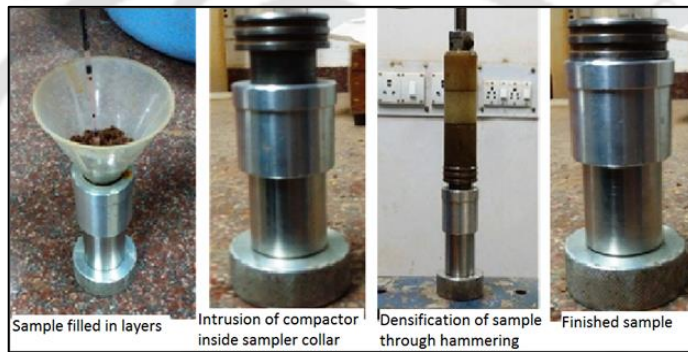
Figure 3.4 Compaction procedure of pin hole sample
