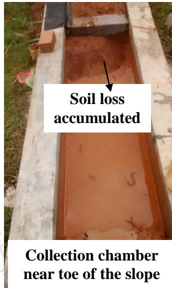
Figure 5.12 Soil loss accumulated in the erosion collection chamber
