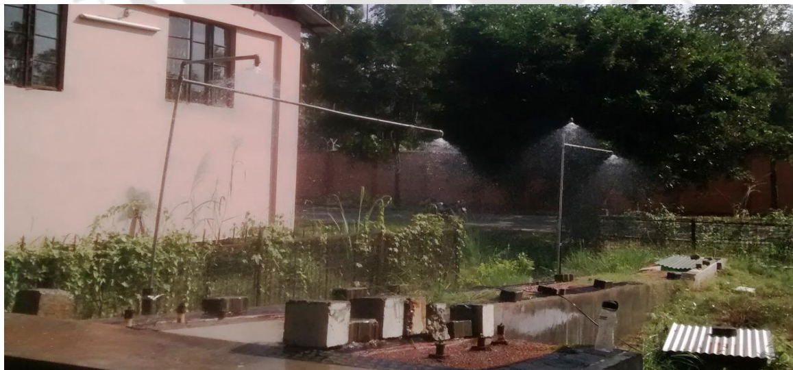
Figure 5.6 Experimental setup for evaluating erosion and infiltration of surface soil in multi-layered cover system
