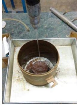
Figure 3.16 Jet impact on the soil surface
