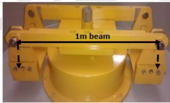
Figure 4.4 Small-scale geotechnical centrifuge facility installed at IIT Guwahati
