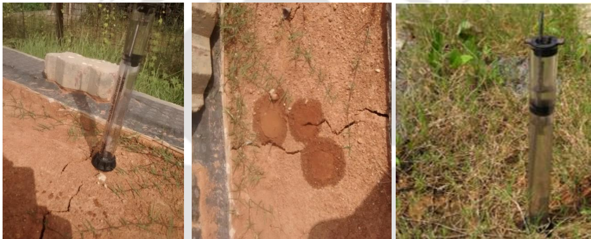
Figure 5.11 Overview of infiltration measurement locations around crack and vegetated area
