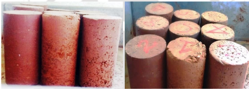
Figure 3.27 Figure depicting oven dried soil samples
