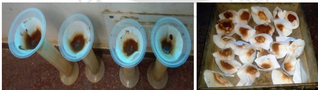
Figure 3.7 Figure depicting the filtration of sediment solutions
