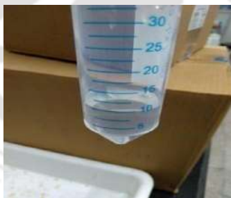
Fig. 4.30 Permeate water obtained following treatment of refinery wastewater in a two-stage STMBR system.
