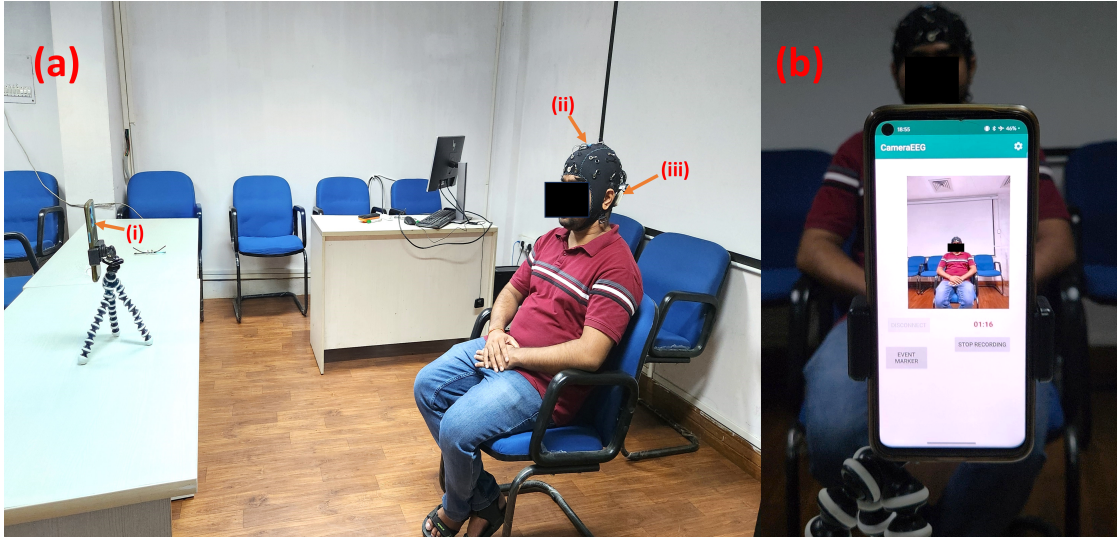
Figure 3.2: (a) The data recording setup for the resting-state eyes-open task, featuring (i) a OnePlus Nord CE 2 Lite 5G smartphone placed on a tripod in front of the subject, (ii) an EasyCap 24-channel EEG cap, and (iii) an mBrainTrain Smarting device mounted on the EEG cap. (b) The CameraEEG Android app running on the smartphone, recording synchronized EEG and video data.
