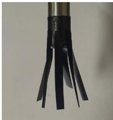
Figure 4.16: Digital photo of the soft gripper used to transfer objects from one location to another
