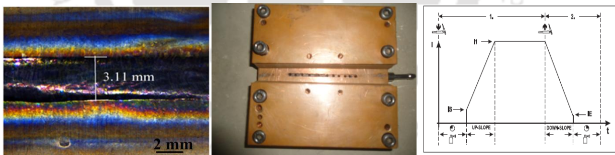
Fig. 4.5 (a) Bead-on-plate welding at 11 A, 4.2 mm/s; (b) Copper fixture used in present investigation; (c) Welding cycle.
