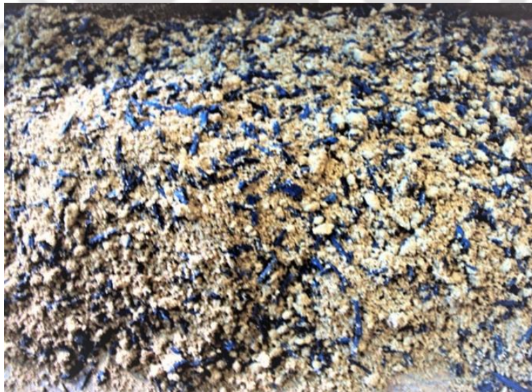
Figure 3.3 Sand-bentonite tire fiber composite
