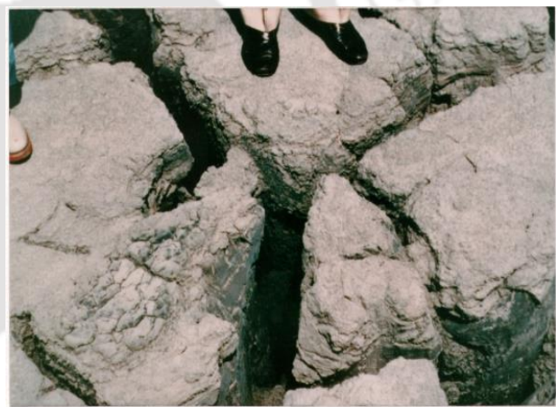
d. A close-up view of the desiccation crack at the hydraulic fill site in Los Angeles (Mitchell 1986)
