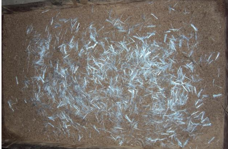
Figure 3.4 Sand–bentonite–fiber composite before mixing
