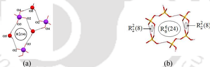
Figure 2.4: (a) R_4^4(12) hydrogen-bond motif in bisulphate-(water) 2 -bisulphate assembly formed within 2.2e (b) Cyclic-hexameric assembly of the dihydrogenphosphate ion of 2.1f .
