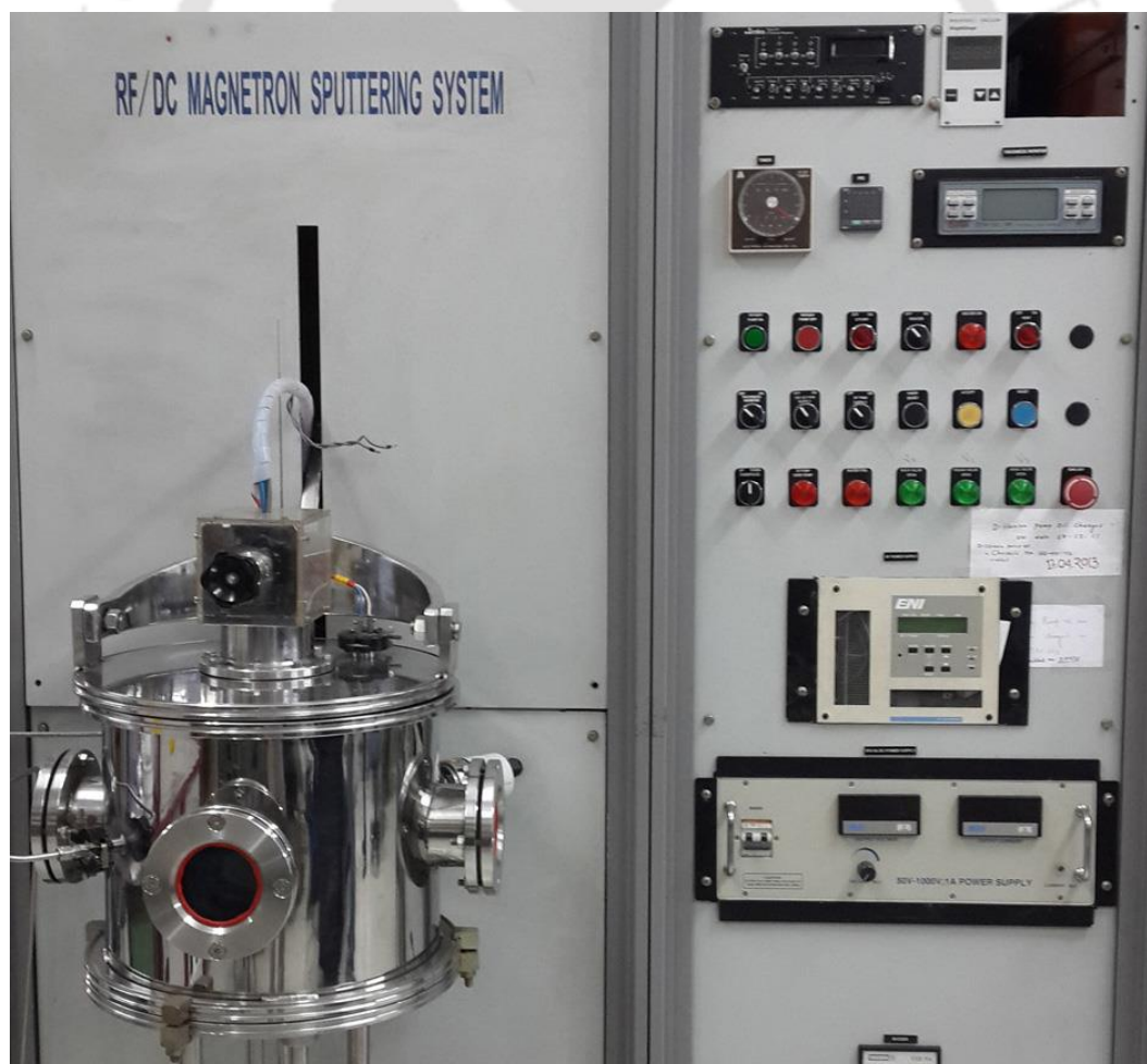
Figure 3.05: Photograph of magnetron sputtering system used in the present work.
