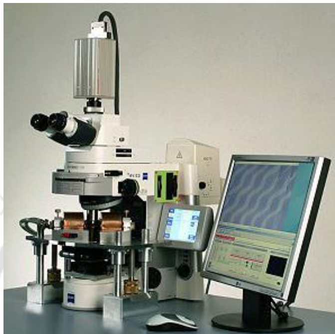
Figure 3.16: Photograph-of the Kerr microscope (Evico Magnetics Ltd. Germany) used in the present study.
