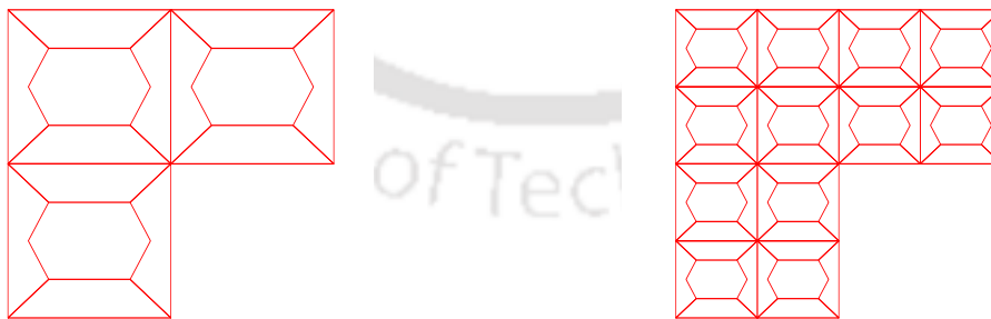
Figure 8.4.9: First 2-levels for the pentagons-quadrilateral mesh for Example 8.4.3.
