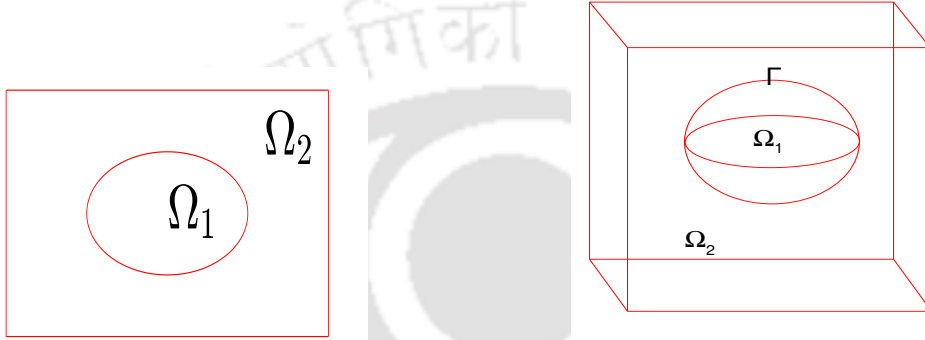
Figure 1.1.1: Domain \Omega and its subdomains \Omega_1, \Omega_2 with interface \Gamma in \mathbb{R}^2 (left) and \mathbb{R}^3 (right).
