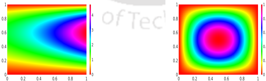
Figure 2.4.4: (Test Example 2.4.2) Component-wise surface plots of WG solution \mathbf{p}_h for WG algorithm. Plot for the first-component of \mathbf{p}_h (left) and plot for second-component of \mathbf{p}_h (right).
