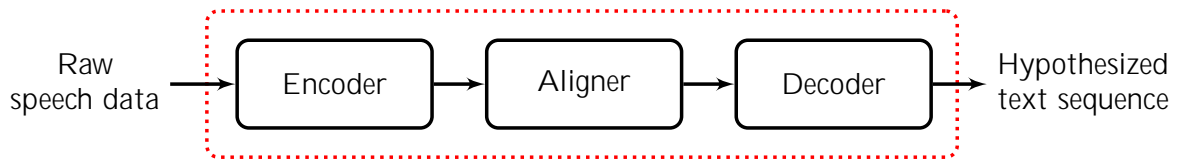
Figure 1.2: Block diagram representing the structure of an E2E ASR framework. All the modules in this framework are jointly optimized with a common objective function.
