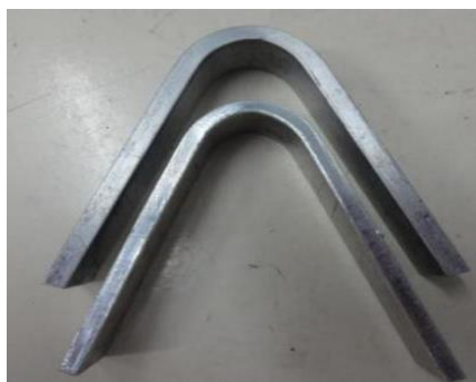
Fig. 7.6. Specimens after bend test
