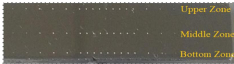
Fig. 3.15. Hardness specimen with indentation marks
