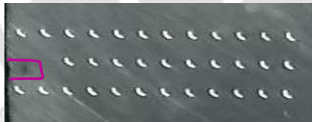
Fig. 5.13. Hardness tested sample after IC test
