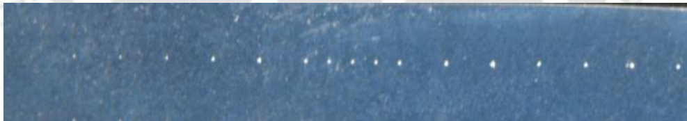
Fig. 6.3. Vickers microhardness tested sample along the weld area after HT
