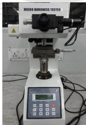
Fig. 3.14. Vickers micro-hardness measuring machine
