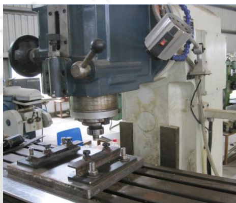
Fig. 3.1. The FSW setup used for the experiments
