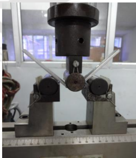
Fig. 3.16. Flexural/bending test setup connected to UTM
