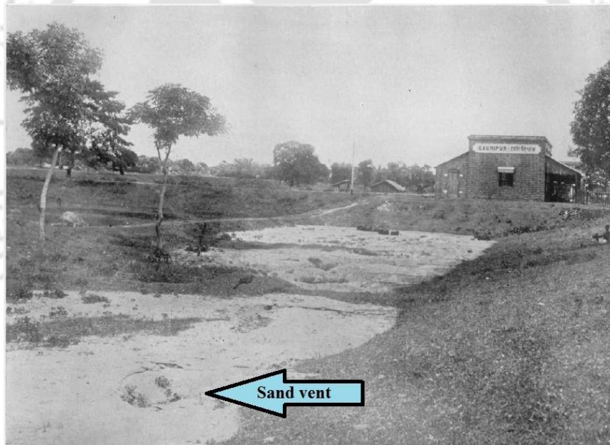
Figure 2.6: Sand vents in Gauripur near Dhubri, Assam after the 1930 Dhubri EQ (modified after Gee 1934)
