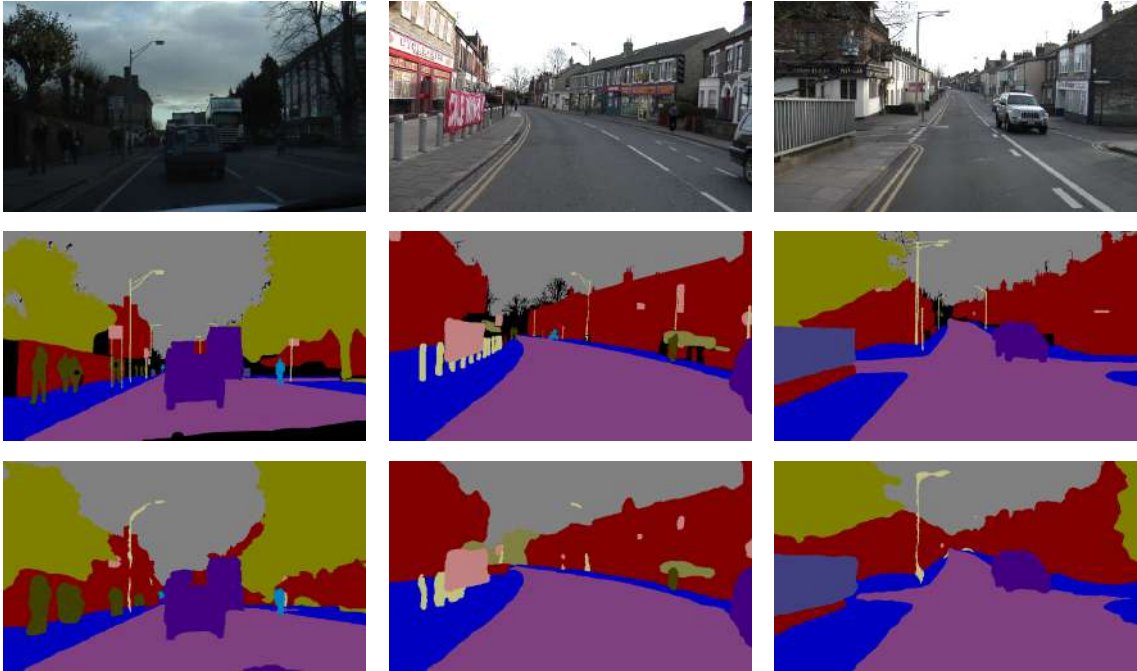
Figure 4.9: Qualitative results: Validation images on the CamVid dataset. First row: Input image; second row: ground truth; third row: BANet output.
