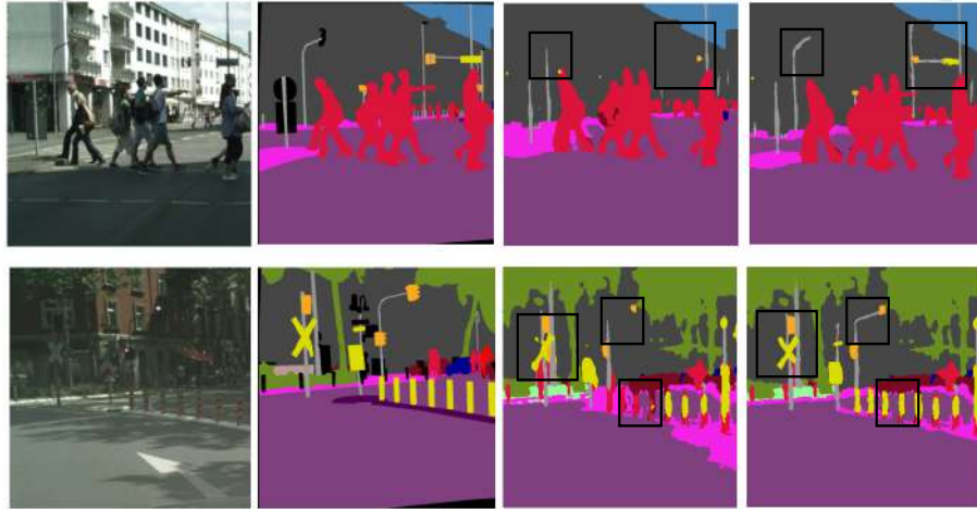
Figure 2.3: Qualitative examples of segmented images produced by the model trained with different loss functions; Column 1: Input Image, Column 2: Ground Truth, Column 3: CE loss(Baseline), Column 4: Dice+CE loss. The improvements in some of the small classes are highlighted in black squares.
