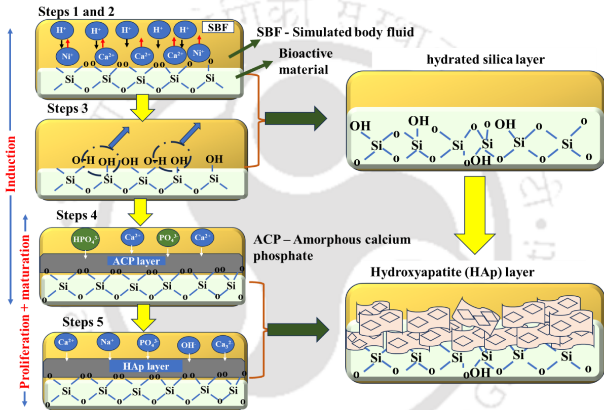
Figure 1.03: Schematic depiction of Hench's ion exchange mechanism [HENC1991, FERR2020] for HAp layer formation on the surface of a bioglass.
