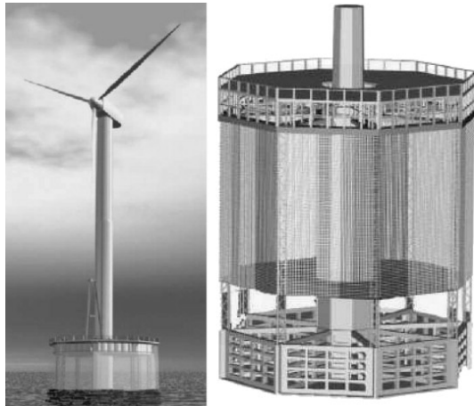
Figure 1.6: Design of the structure composed by the aerogenerator and the aquaculture cage. Courtesy of INR Eólica. [4]
