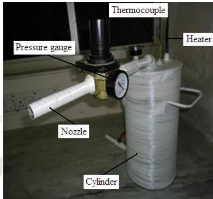
Fig. 6.1: Laboratory set up for insulated solid cylinder with pressure gauge, heater and thermocouple
