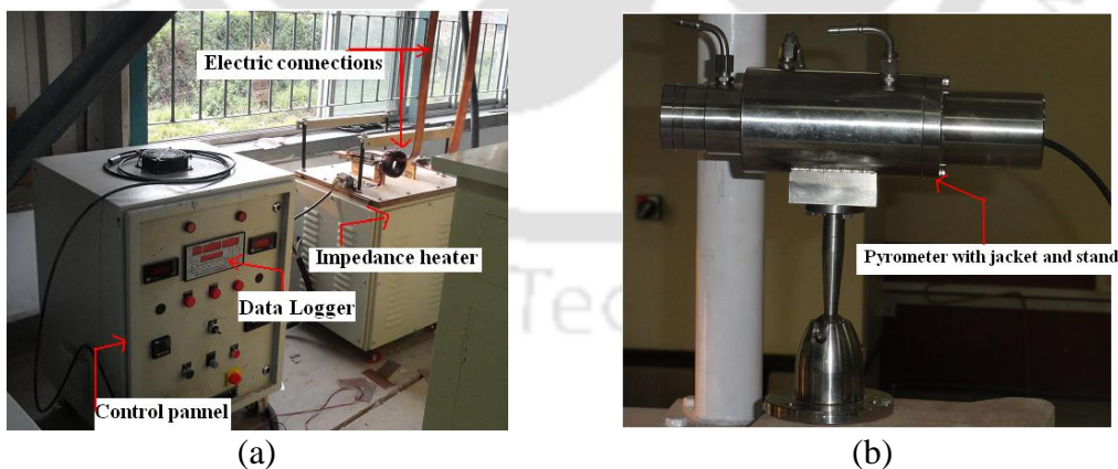
Figure 3.10. Photographs of (a) impedance heating system and (b) non-contact IR pyrometer.
