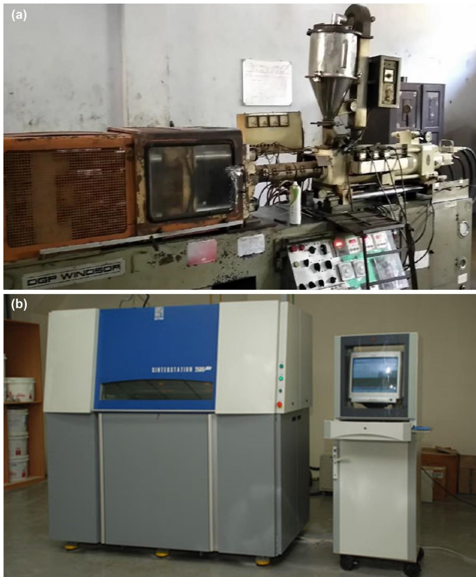
Fig. 3.3 (a) Windsor GT-50 injection-molding machine and (b) Sinterstation 2500 selective laser sintering machine.
