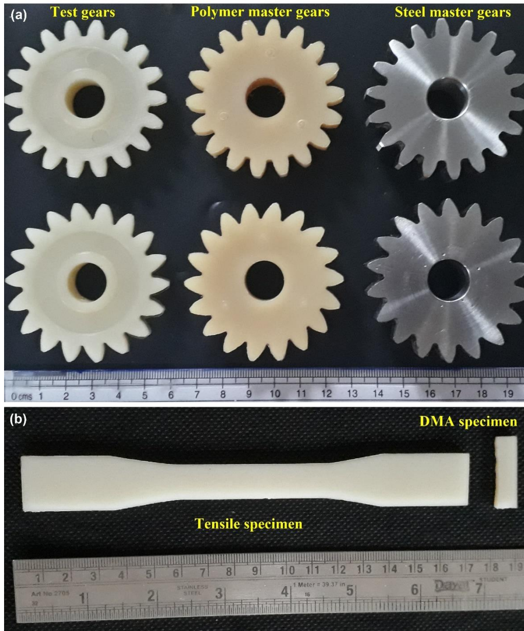
Fig. 3.2 (a) Symmetric and asymmetric master and test gears and (b) Tensile specimen used in monotonic tests and flexure specimen used in DMA.
