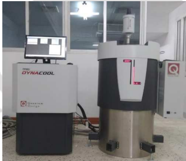
Figure 2.30. Photograph of the 9T PPMS (Quantum Design, DynaCool) with a VSM insert.
