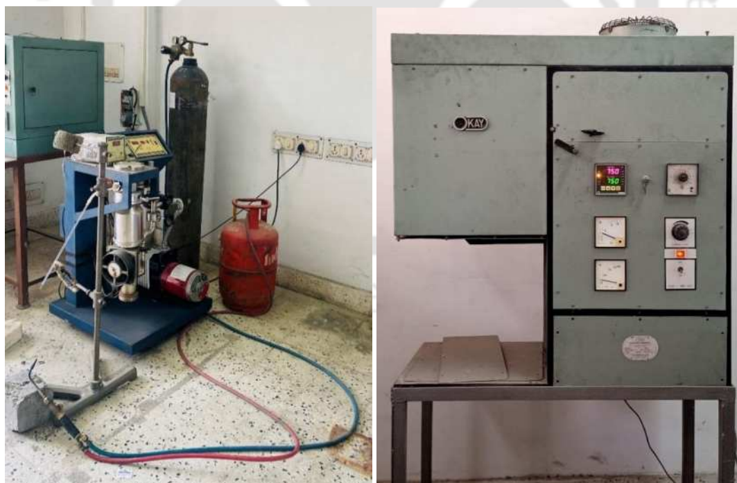
Figure 2.04. Ampoule vacuum sealing setup (left) and the raising hearth furnace (right) used for processing as-melted bulk Heusler alloy ingot.
