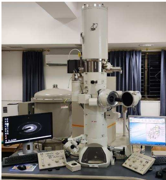
Figure 2.24. Photograph of JEOL-2100F TEM utilized in this work.
