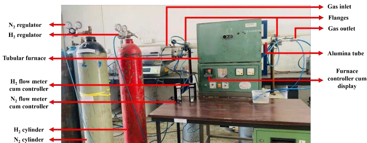
Figure 2.02. Tubular furnace along with the gas manifold used for processing the nanoparticles.
