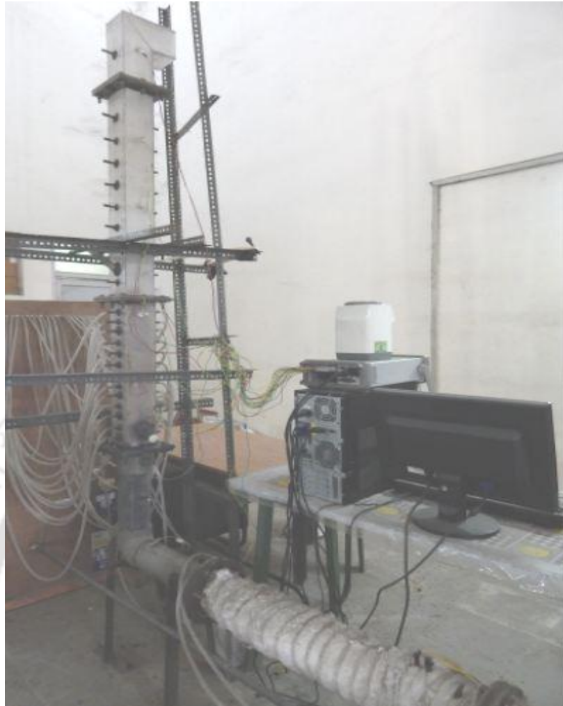
Fig. 3.2(b) Photographs of bubbling fluidized bed drier at \theta = 0^\circ inclination (vertical bed)
