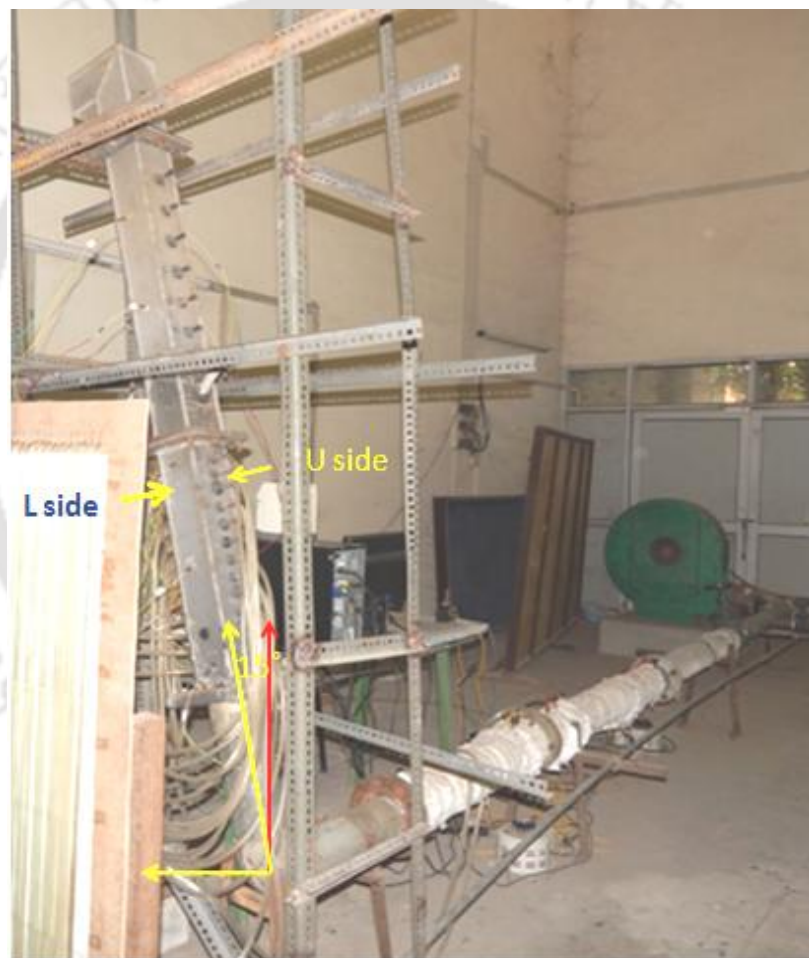
Fig. 3.2(a) Photographs of bubbling fluidized bed drier at \theta = 15^\circ
