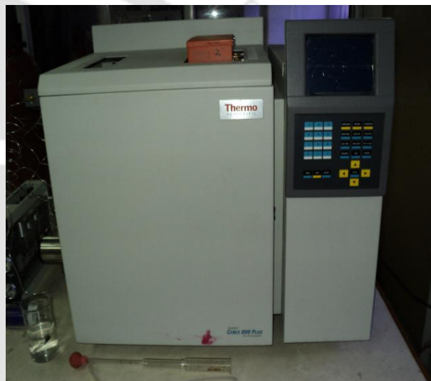
Fig. IV.7 Gas Chromatography machine
