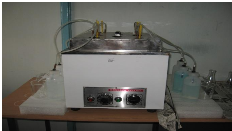
Fig. IV.1 Water bath where small scale digesters were kept for fermentation under constant temperature condition
