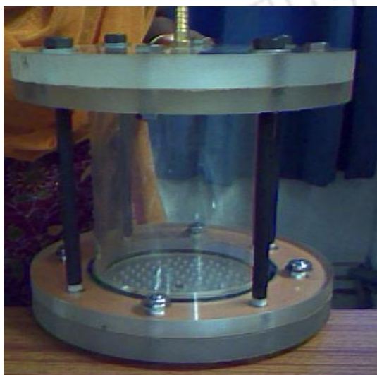
Fig. 6.5 The scrubber after assembling (vertical position)
