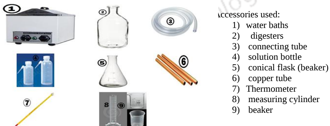
Fig. IV.3 Various accessories used in the experimental set-up:
