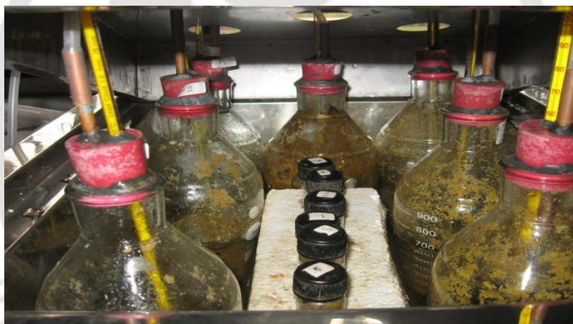
Fig. IV.2 Small scale digesters inside water bath kept for fermentation
