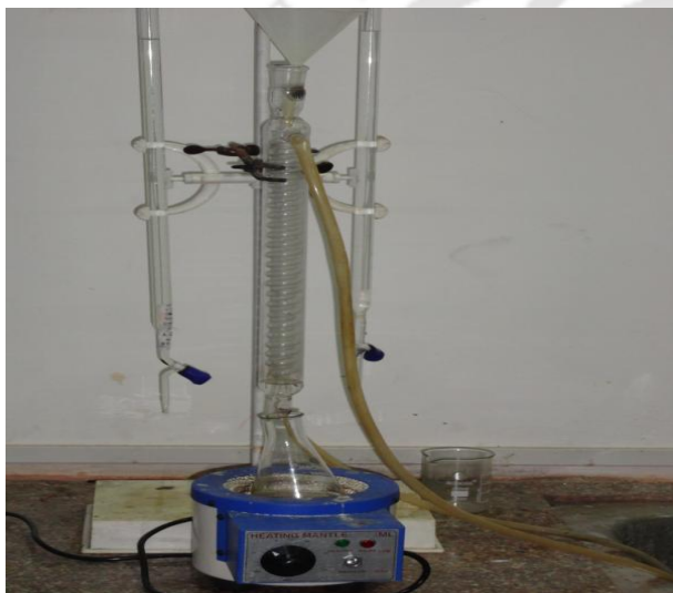
Fig. IV.6 Set-up for COD with heating mantle
