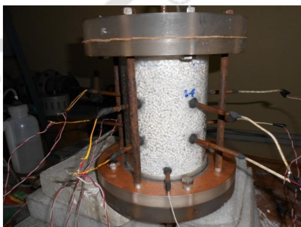
Fig. 6.9 Biogas passed through the scrubber
