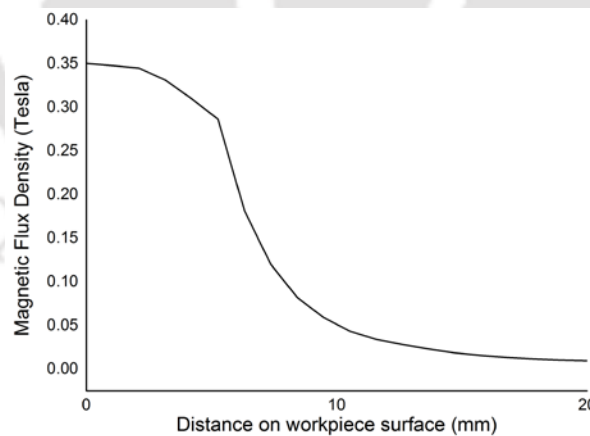
Fig. 2.5 Distribution of magnetic flux density along line AB (Fig. 2.1(a)) for 1 st configuration on workpiece surface
