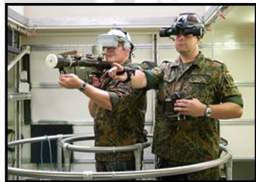
Figure 2.13: Virtual reality trainer used for STRIGER crew training (Cassidian - Virtual Military Training Systems, 2012)
