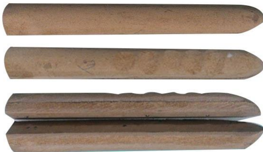
Figure 5.5: Wood pattern for making the modified stylus from plastic
