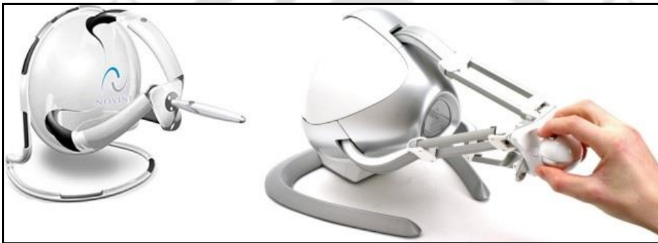
Figure 3.12: Falcon haptic device with ball and pen type manipulator (“Novint Falcon,” 2007)
