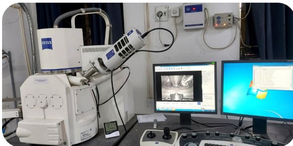
Figure 2.09. Field emission scanning electron microscope (Zeiss, Sigma) with EDS unit.
