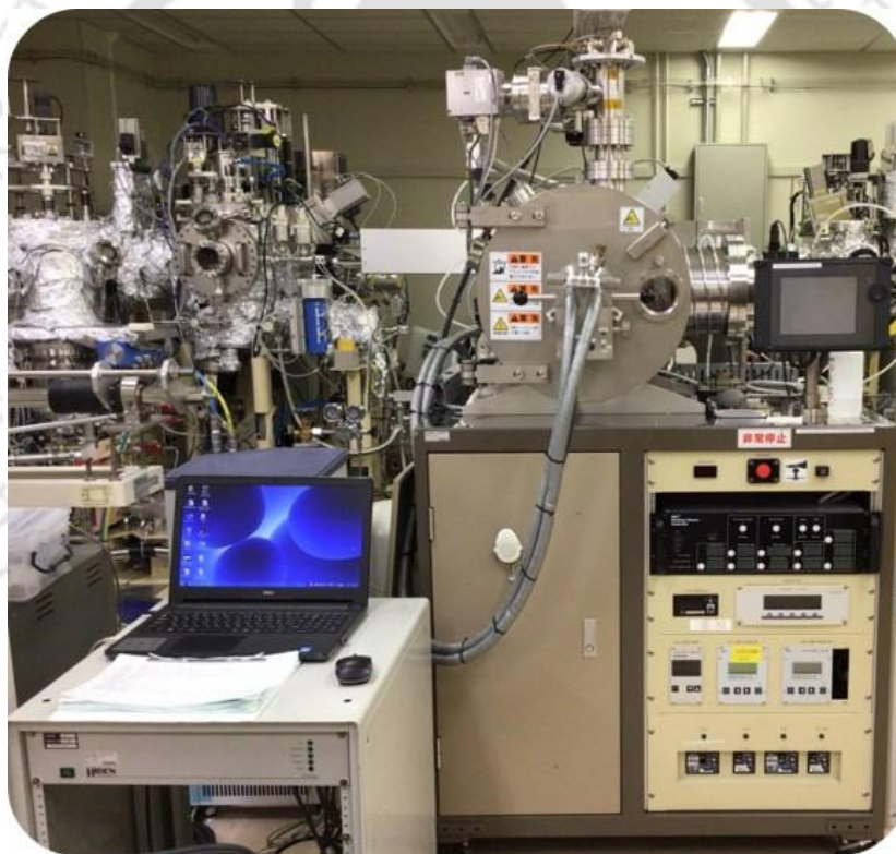
Figure 2.07. An Ar ion milling setup is used to etch and deposit thin film devices.
