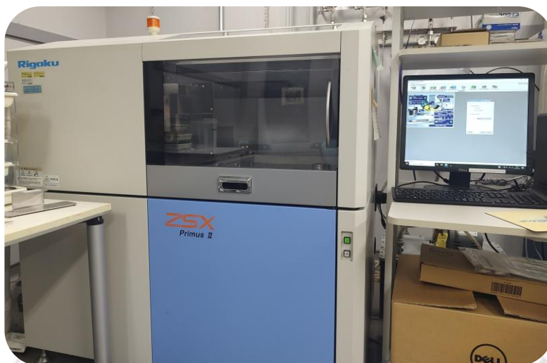
Figure 2.11. Photograph of the XRF instrument used for elemental analysis of thin film.
