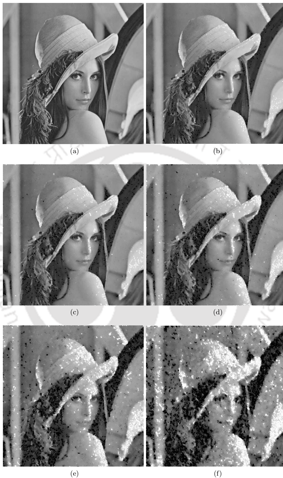
Fig. 3.6: (a) Original image. The output of the proposed reconstruction filter for the “Lena” image corrupted with (b) 50% (c) 60% (d) 70% (e) 80% and (f) 90% random-valued impulse noise, respectively. The detection stage of the SD-ROM filter is applied for the detection of the impulse locations.
