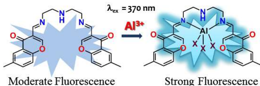
Scheme 6B.2 Plausible binding mechanism of L 10 towards Al^{3+} in aqueous medium.
